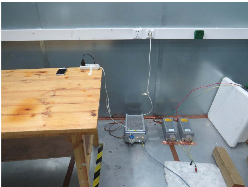
Picture 3 Conducted Emission Test Setup
