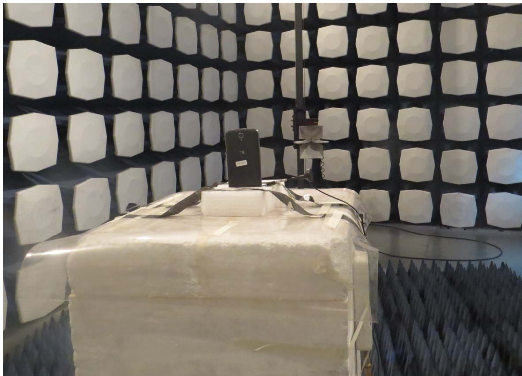
Picture 2 Radiated Spurious Emissions Test Setup
