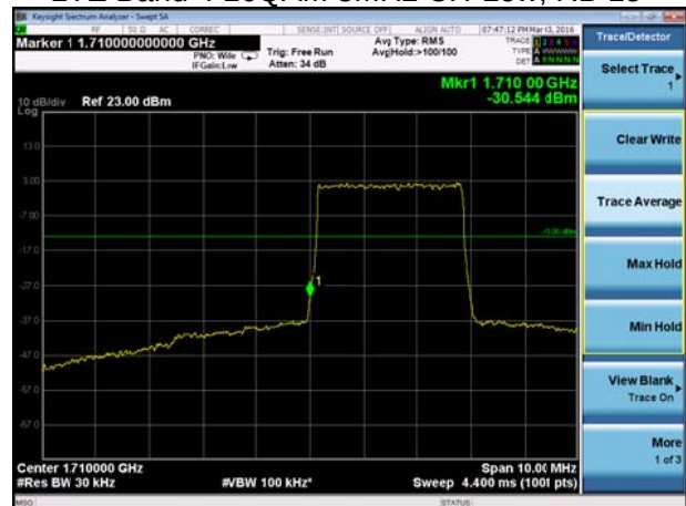
LTE Band 4 16QAM 3MHz CH-Low, RB 15
