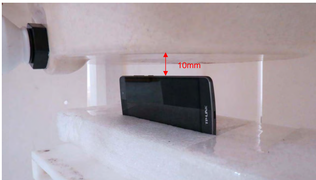
Picture 21: Right Side, the distance from handset to the bottom of the Phantom is 10mm
