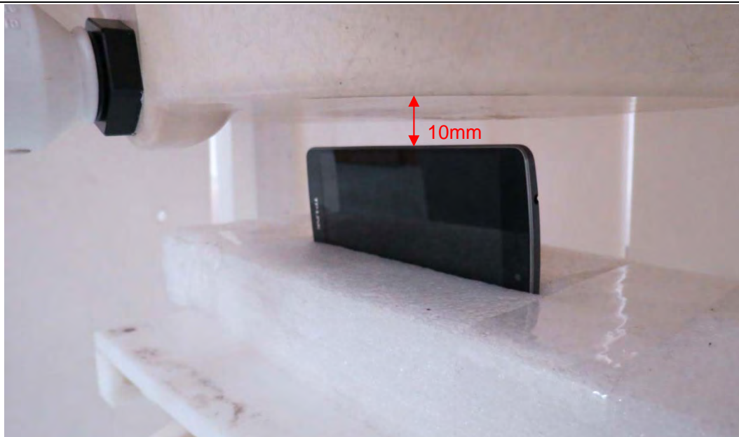
Picture 20: Left Side, the distance from handset to the bottom of the Phantom is 10mm
