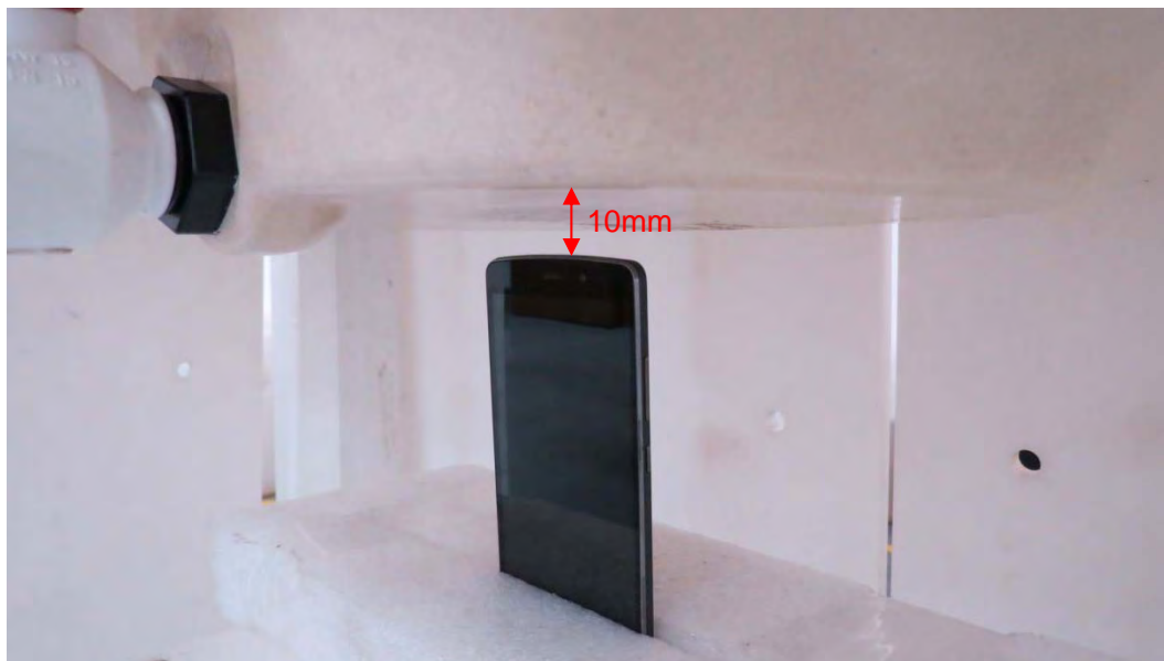
Picture 22: Top Side, the distance from handset to the bottom of the Phantom is 10mm
