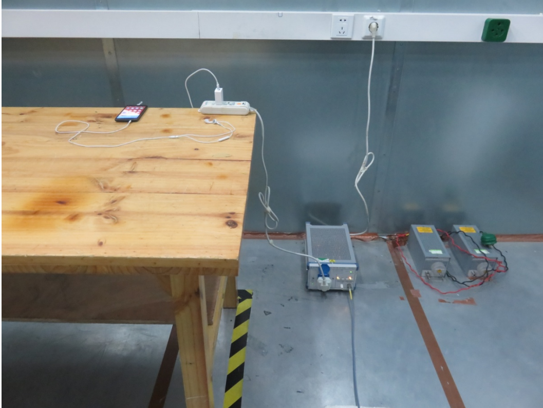
Picture 3 Conducted Emission Test Setup
