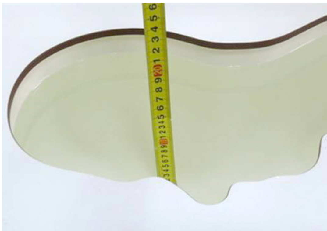
Picture 6: liquid depth in the head Phantom (1750 MHz, 15.3cm depth)
