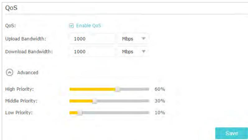
The screenshot shows the 'QoS' configuration page. At the top, 'Enable QoS' is checked. Below that, 'Upload Bandwidth' and 'Download Bandwidth' are both set to 1000 Mbps. Under the 'Advanced' section, there are three priority levels: 'High Priority' at 60%, 'Middle Priority' at 30%, and 'Low Priority' at 10%. A 'Save' button is located at the bottom right of the form.
