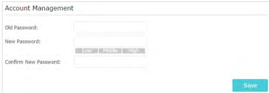
The screenshot shows the 'Account Management' section of the TP-Link web interface. It includes fields for 'Old Password', 'New Password' (with a strength indicator from 'Low' to 'High'), and 'Confirm New Password'. A 'Save' button is located at the bottom right.
