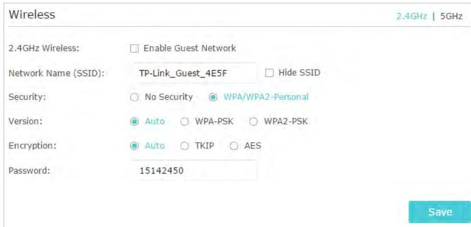
The screenshot shows the 'Wireless' configuration page for a 2.4GHz guest network. The page has a header with 'Wireless' and '2.4GHz | 5GHz' buttons. The configuration fields are as follows:
