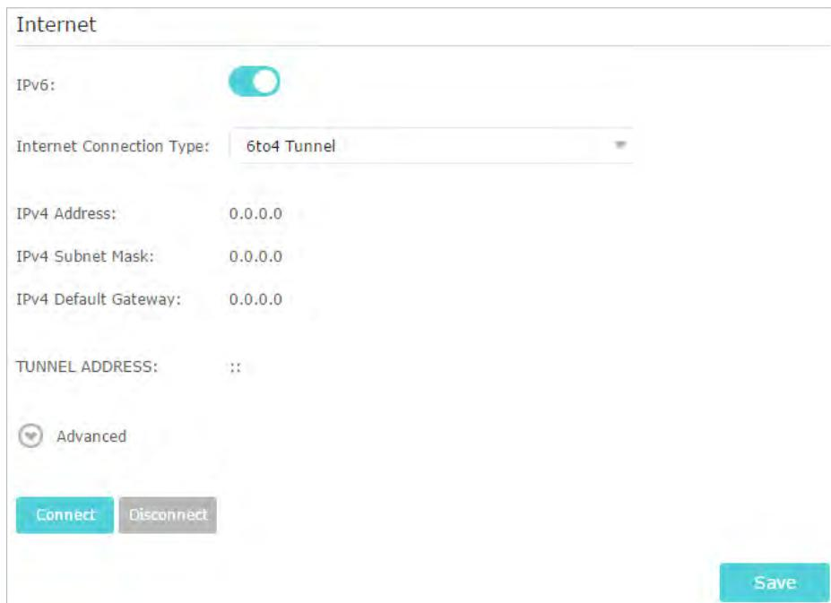
The screenshot shows the 'Internet' configuration page. The 'IPv6' toggle switch is turned on. The 'Internet Connection Type' dropdown is set to '6to4 Tunnel'. Below it are fields for 'IPv4 Address' (0.0.0.0), 'IPv4 Subnet Mask' (0.0.0.0), and 'IPv4 Default Gateway' (0.0.0.0). The 'TUNNEL ADDRESS' field is empty. There is an 'Advanced' link with a gear icon. At the bottom are 'Connect' and 'Disconnect' buttons, and a 'Save' button.
