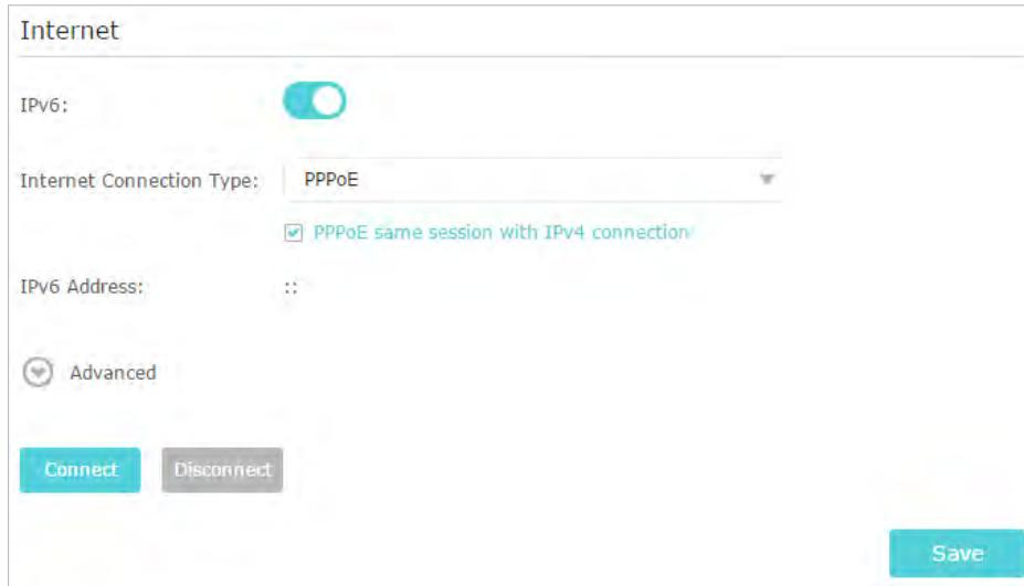
The screenshot shows the 'Internet' configuration page. The 'IPv6' toggle switch is turned on. The 'Internet Connection Type' dropdown is set to 'PPPoE'. A checked checkbox below it says 'PPPoE same session with IPv4 connection'. The 'IPv6 Address' field is empty. There is an 'Advanced' link with a gear icon. At the bottom are 'Connect' and 'Disconnect' buttons, and a 'Save' button.
