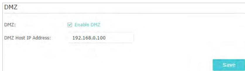
The screenshot shows a configuration interface for a TP-Link router. The top bar has 'DMZ' in bold. Below it, there's a section for 'DMZ' with a checked checkbox labeled 'Enable DMZ'. Underneath, there's a 'DMZ Host IP Address' field containing '192.168.0.100'. At the bottom right of the interface is a blue 'Save' button.
