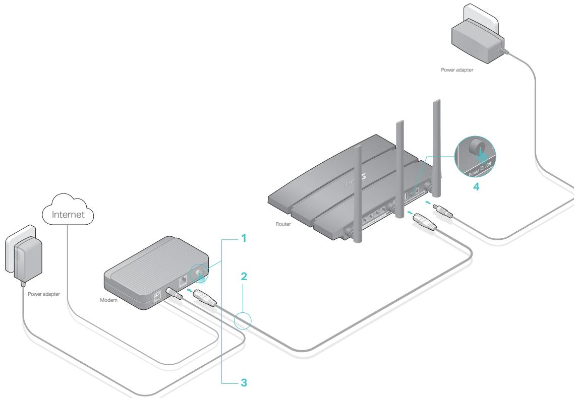
1. Turn off the modem, and remove the backup battery if it has one.
