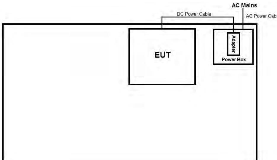
**Test Setup Diagram – Radiated Emission Test**
