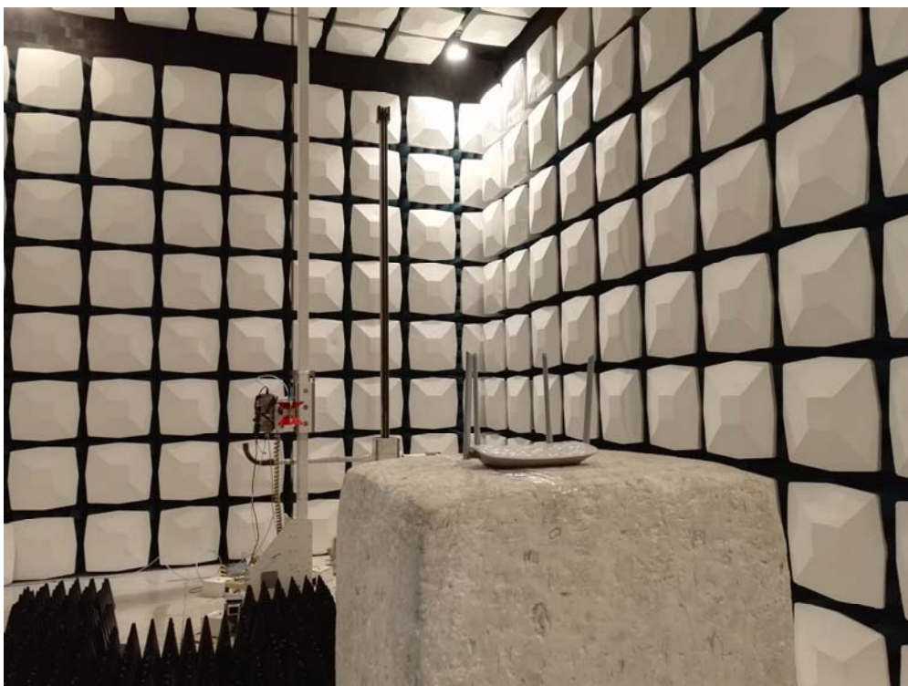
Description: Radiated Emission Test Setup for 1~18GHz
