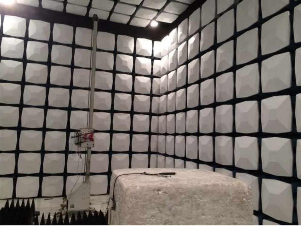
Description: Radiated Emission Test Setup for 1~18GHz
