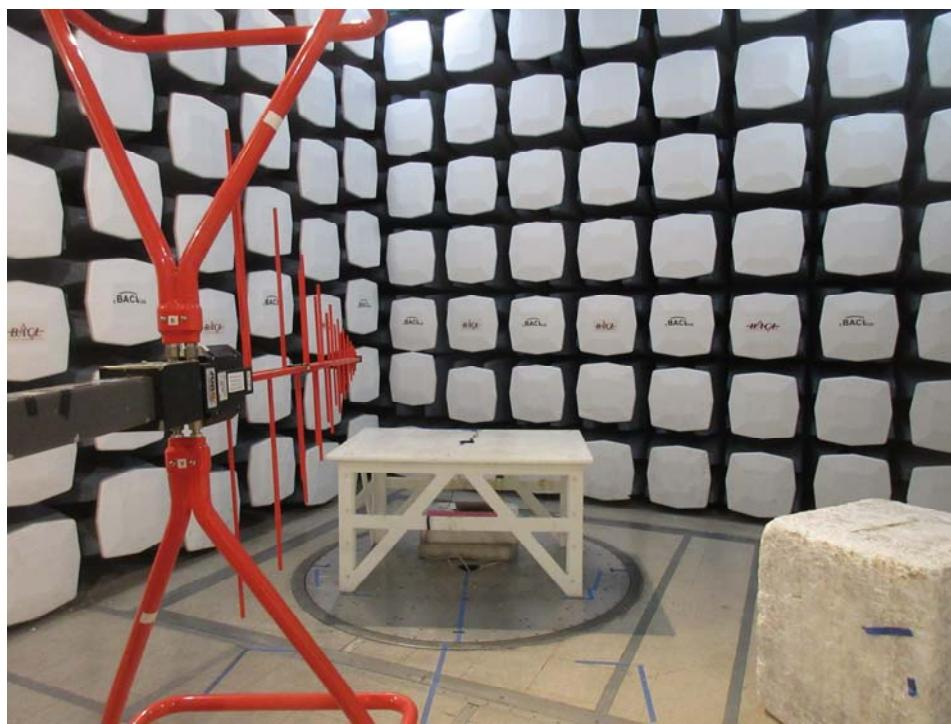
**1.6 Radiated Spurious Emissions: 30MHz - 1GHz Rear View at 3 meters**
