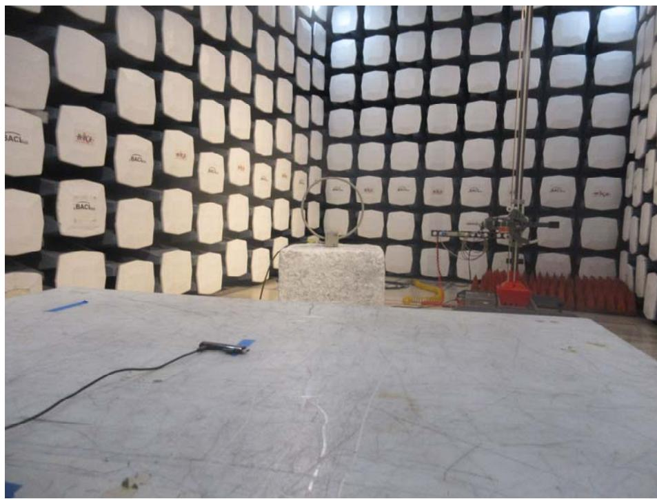
**1.5 Radiated Spurious Emissions: 30MHz - 1GHz Front View at 3 meters**
