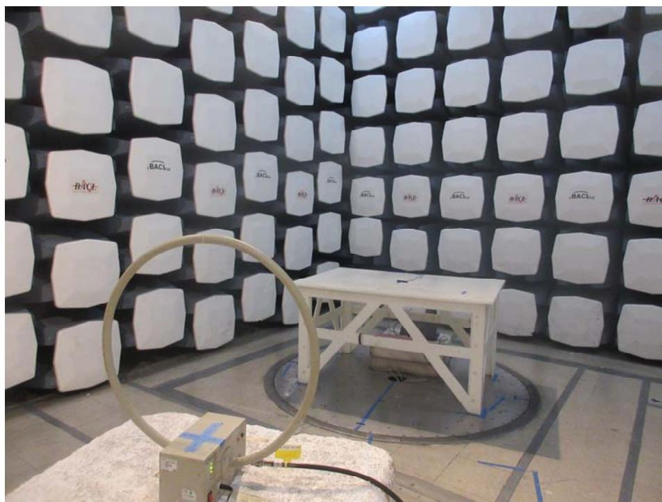
**1.4 Radiated Spurious Emissions: 9kHz – 30MHz Perpendicular Rear View at 3 meters**
