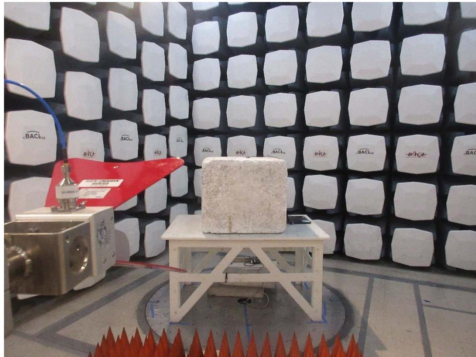
**1.8 Radiated Spurious Emissions: 1-18 GHz Rear View at 1 meter**
