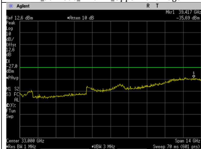
U-NII-2A_5300MHz_high_Mid Ch_60_20MHz BW_a- mode_-27dBm_26-40GHz
