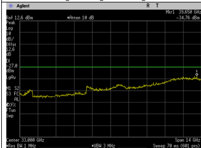
U-NII-3_5795MHz_High_Mid Ch_159_40MHz BW_n/ac-mode_-27dBm_26-40GHz_Peak
