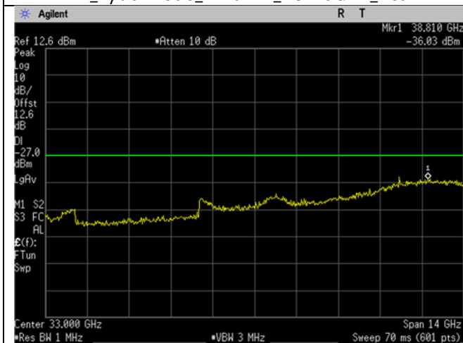
U-NII-3_5825MHz_High Ch_165_20MHz BW_a-mode_-27dBm_26-40GHz_Peak
