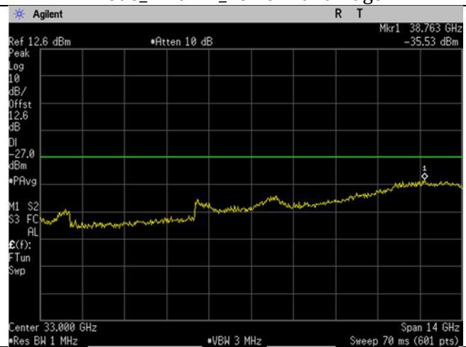
U-NII-2C_5590MHz_Mid Ch_118_40MHz BW_n/ac-mode_-27dBm_26-40GHz
