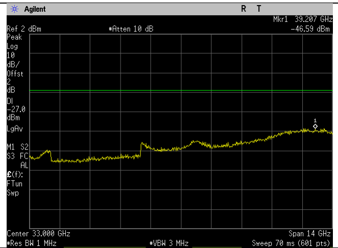
U-NII-3_5785MHz_Mid Ch_157_20MHz BW_a-mode_-27dBm_26-40GHz_Peak_Port 2
