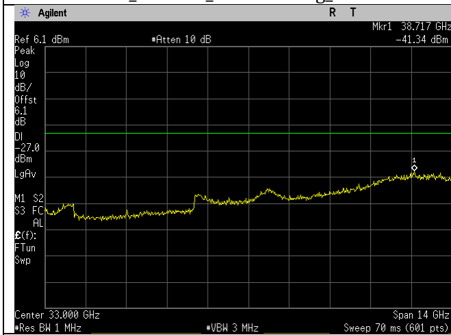
FCC_U-NII-1_5190MHz_Low_Ch_38_40MHz_BW_n-mode_-27dBm_26-40GHz_Port 1
