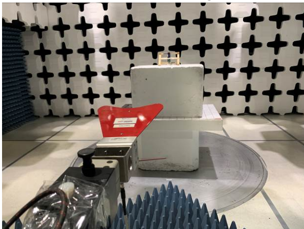
Radiated Emission Test Above 1GHz Front View
