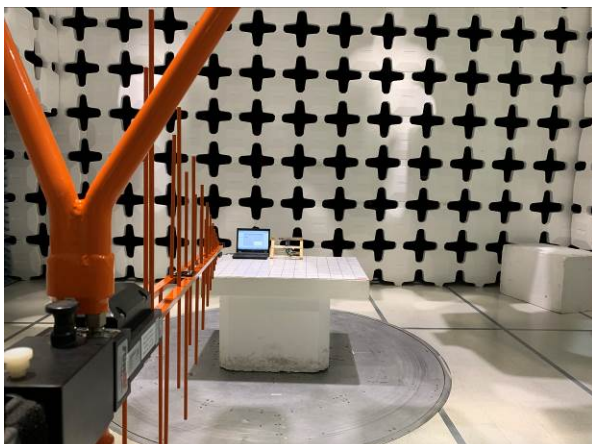
Radiated Emission Test below 1GHz Front View
