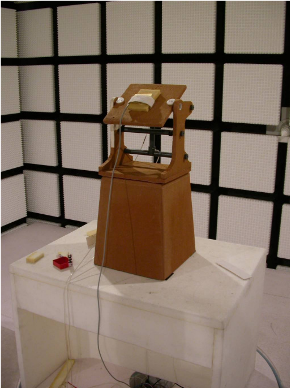
Spurious emission measurement 1 GHz – 12 GHz
