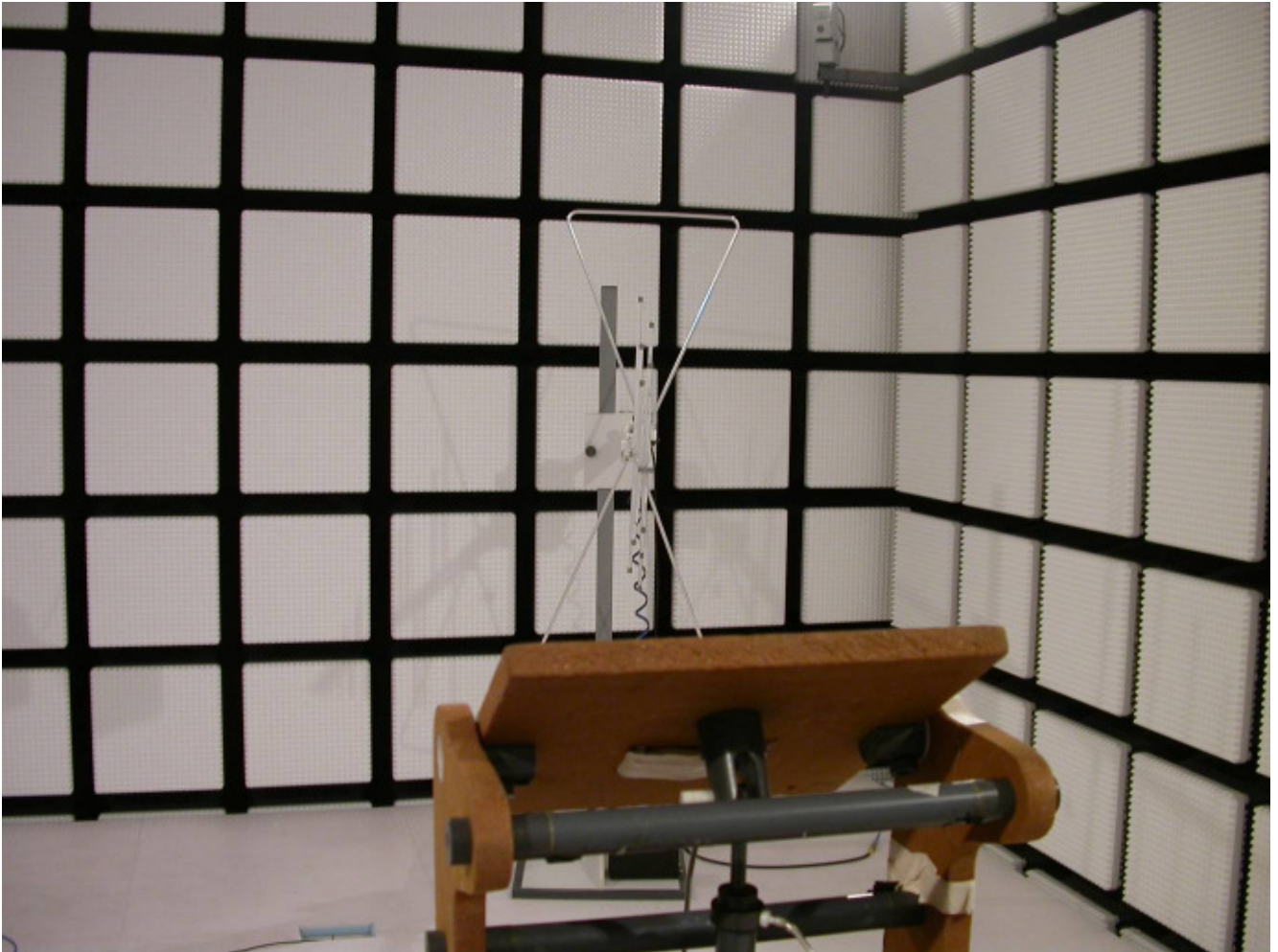
Spurious emission measurement 1 GHz – 12 GHz
