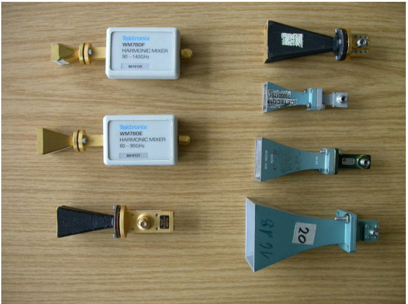
Spurious emission measurement equipment 12 GHz – 110 GHz
