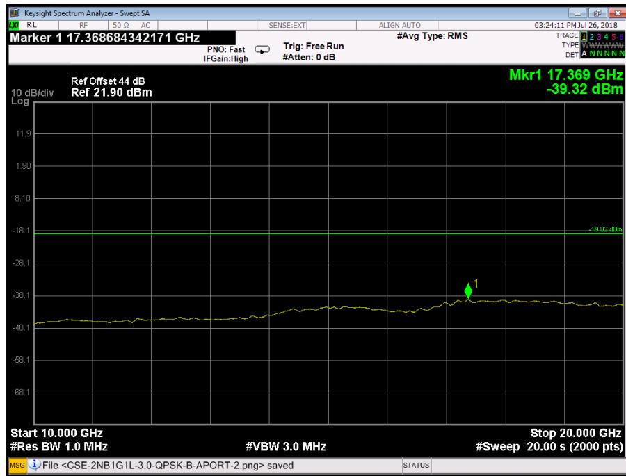
Port A, Channel Position M, LTE 3.0 MHz
