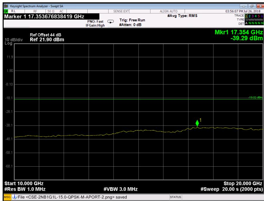
Port A, Channel Position T, LTE 15.0 MHz
