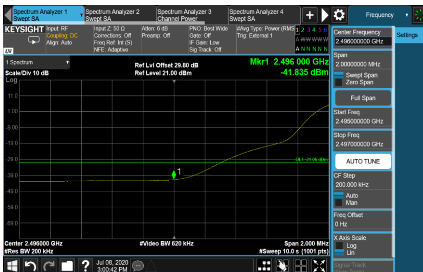
Port 56, Channel Position B, LTE 20.0MHz
