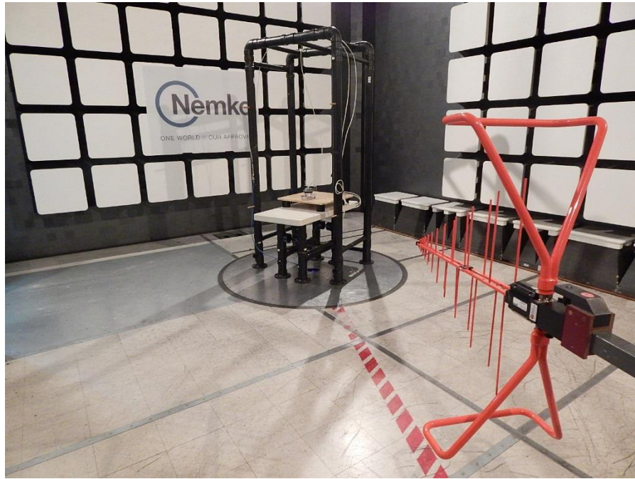
Figure 7.1-19: Radiated emissions setup photo
