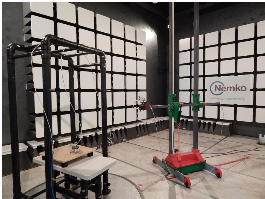
Figure 7.1-21: Radiated emissions setup photo
