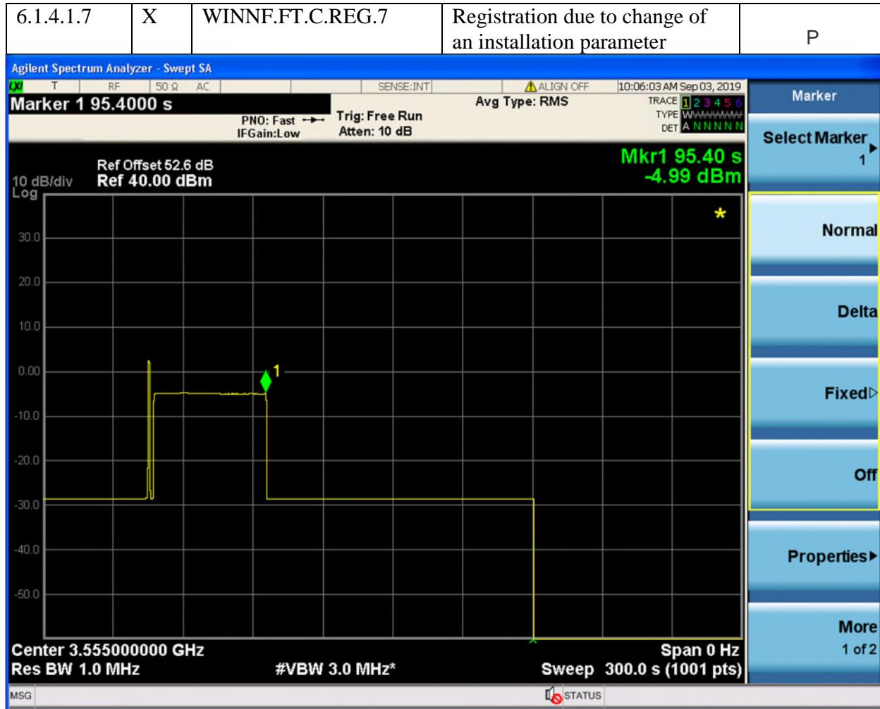
Test Harness logs and timing on graph was verified, the EUT passed the requirement.
