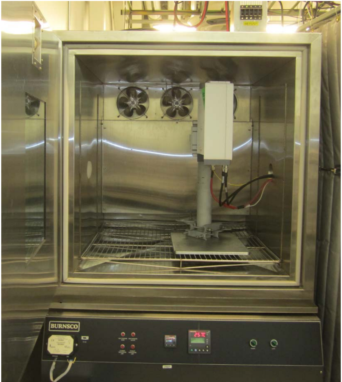
Figure 3.6-2: EUT Set-up for Radio Compliance Testing
