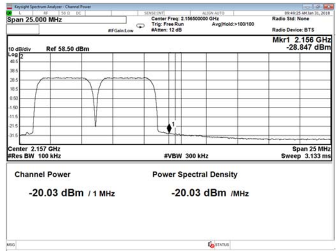
Figure 8.2-34: Conducted band edge emission at 2181 MHz, Ant B, QPSK, 2-carrier operation (RBW = 1 MHz)
