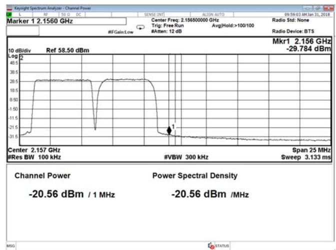
Figure 8.2-36: Conducted band edge emission at 2181 MHz, Ant A, QPSK, multi-RAT operation LTE and WCDMA (RBW = 1 MHz)
