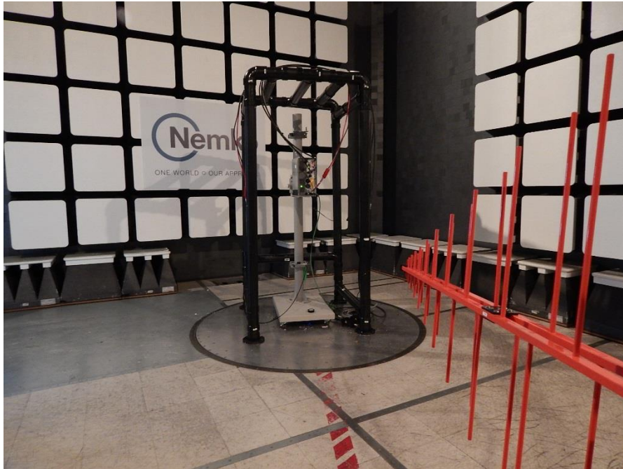
Figure 8.3-2: EUT Set -up for Radiated Compliance Testing – below 1 GHz
