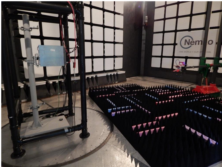
Figure 8.3-3: EUT Set -up for Radiated Compliance Testing– above 1 GHz
