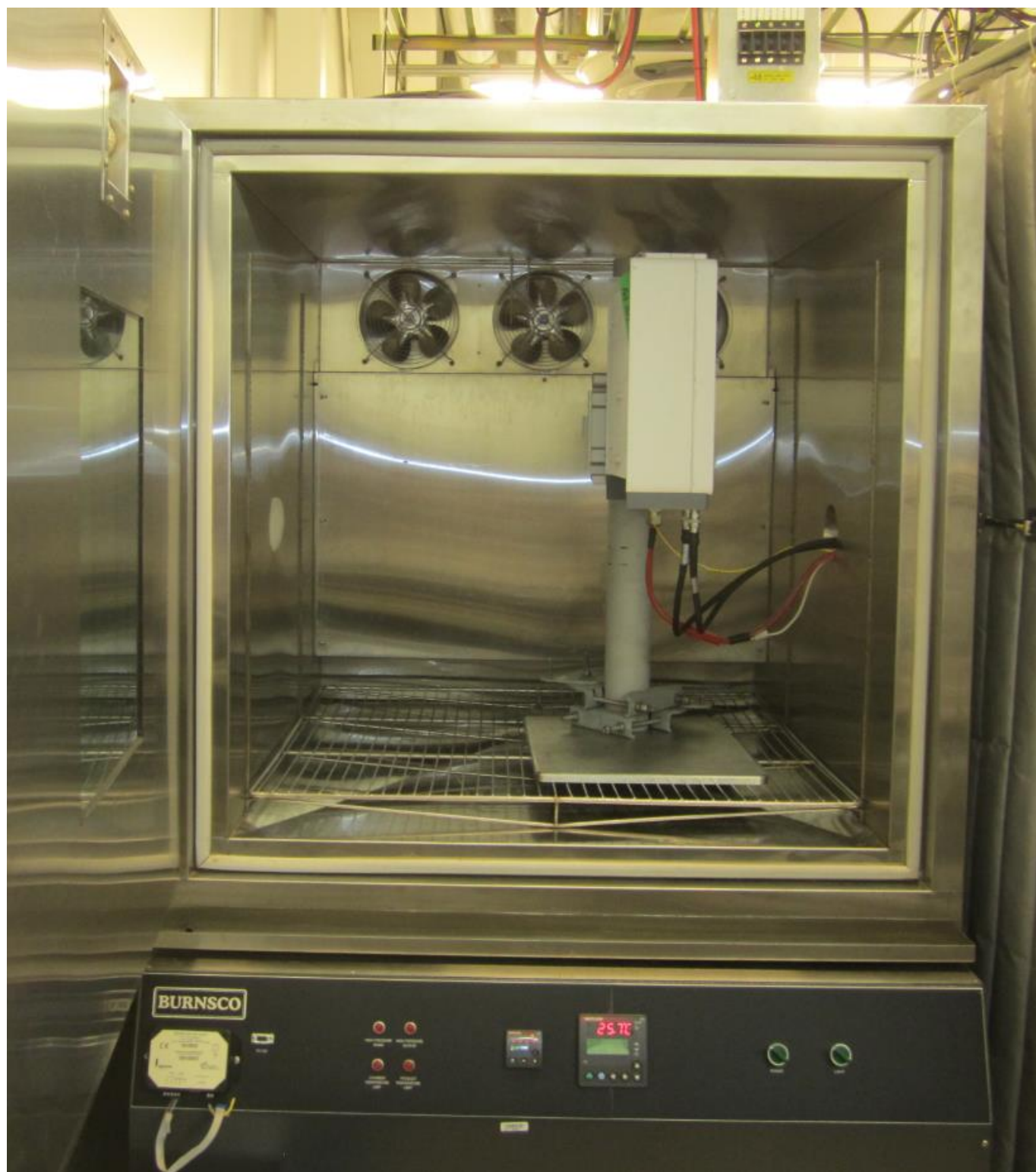
Figure 3.6-2: EUT Set-up for Radio Compliance Testing
