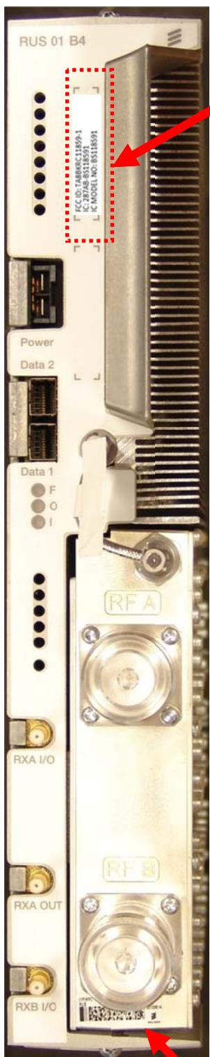
The FCC and IC ID label is located on the front.
