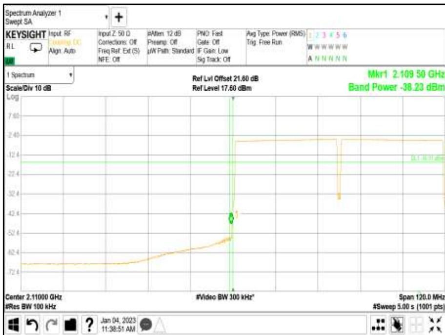
Antenna Port A A - Modulation NR30+NR30: QPSK - Carrier Bandwidth 30+30 MHz - Channel Position T
