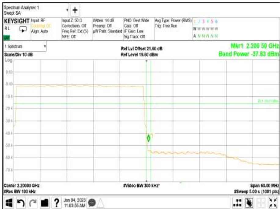
Antenna A - Modulation NR: QPSK - Carrier Bandwidth NR: 40.0 MHz - Channel Position B
