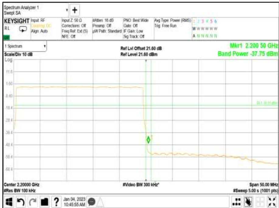
Antenna A - Modulation NR: QPSK - Carrier Bandwidth NR: 30.0 MHz - Channel Position B
