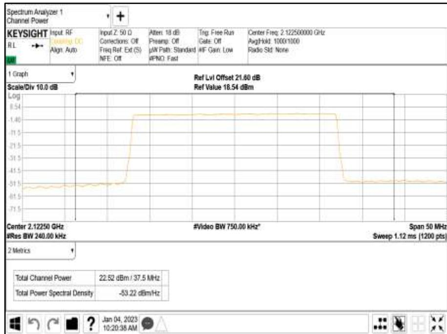
Antenna Port A Pk-Av Ratio - Modulation NR: QPSK - Carrier Bandwidth 25.0 MHz - Channel Position B
