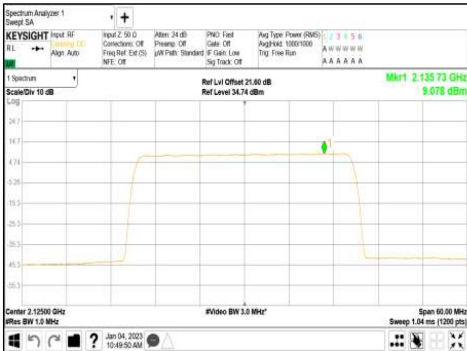
Antenna Port A Carrier Power - Modulation NR: QPSK - Carrier Bandwidth 40.0 MHz - Channel Position B
