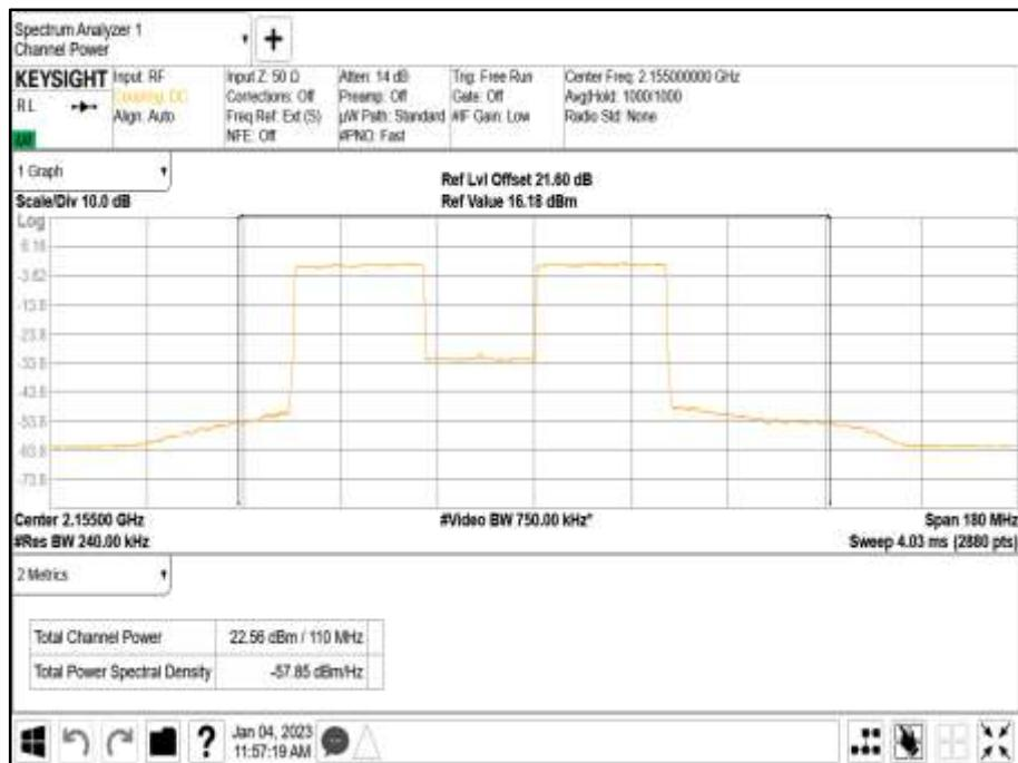
Antenna Port B Carrier Power - Modulation \* NR30+NR30: QPSK - Carrier Bandwidth 30+30 MHz - Channel Position B
