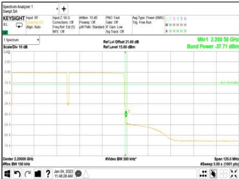
Antenna Port A A - Modulation \* NR25+NR25: QPSK - Carrier Bandwidth 25+25 MHz - Channel Position B
