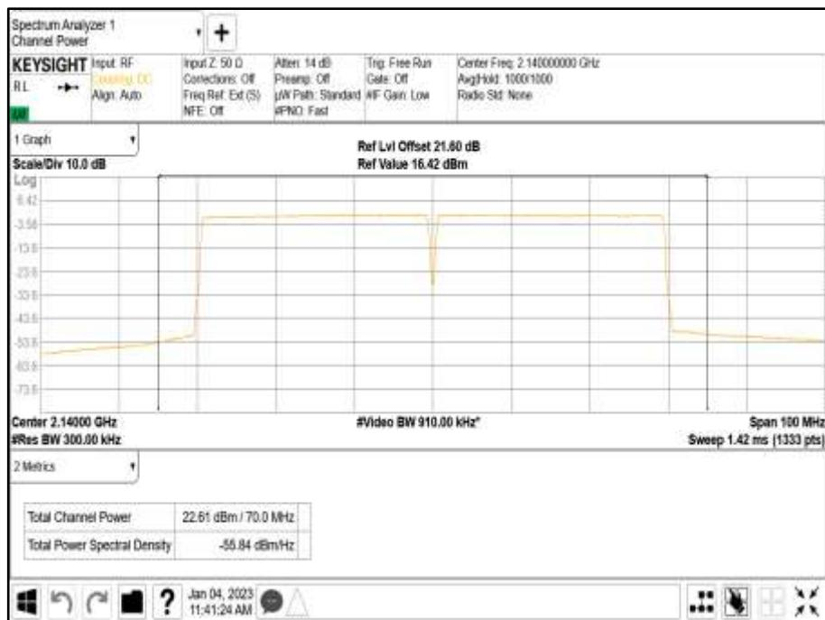
Antenna Port B Carrier Power - Modulation \* NR25+NR25: QPSK - Carrier Bandwidth 25+25 MHz - Channel Position B
