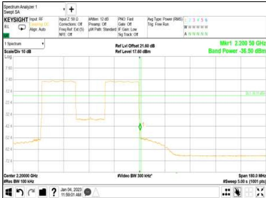
Antenna Port A A - Modulation \* NR30+NR30: QPSK - Carrier Bandwidth 30+30 MHz - Channel Position B
