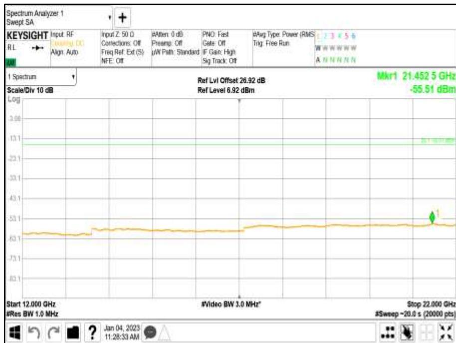
Antenna A - Modulation \* NR25+NR25: QPSK - Carrier Bandwidth 25+25 MHz - Channel Position B - Band 1 - Range 0.009 to 4000 MHz
