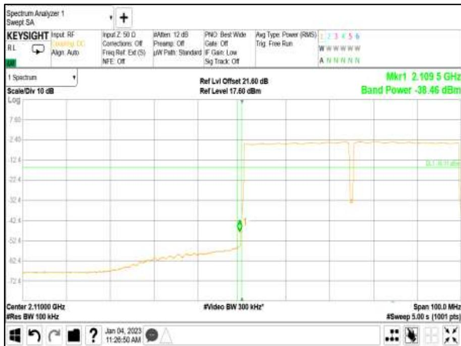
Antenna Port A A - Modulation NR25+NR25: QPSK - Carrier Bandwidth 25+25 MHz - Channel Position T
