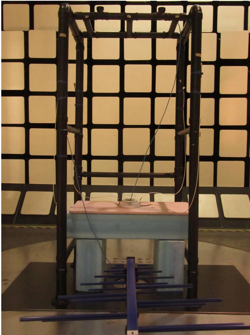
Figure 39: EUT Setup for RE tests at 30 MHz to 1 GHz
