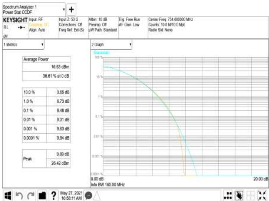
Antenna Port A PSD - Modulation LTE: QPSK - Carrier Bandwidth 10.0 MHz - Channel Position B
