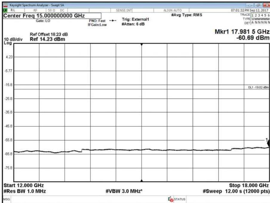
Antenna B - LTE Modulation QPSK - LTE Carrier Bandwidth 10.0 MHz - Channel Position B - Band 4 - Range 18000 to 27000 MHz
