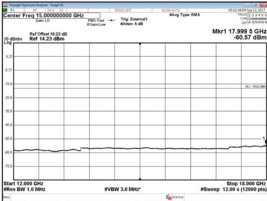
Antenna A - LTE Modulation QPSK - LTE Carrier Bandwidth 20.0 MHz - Channel Position B - Band 4 - Range 18000 to 27000 MHz
