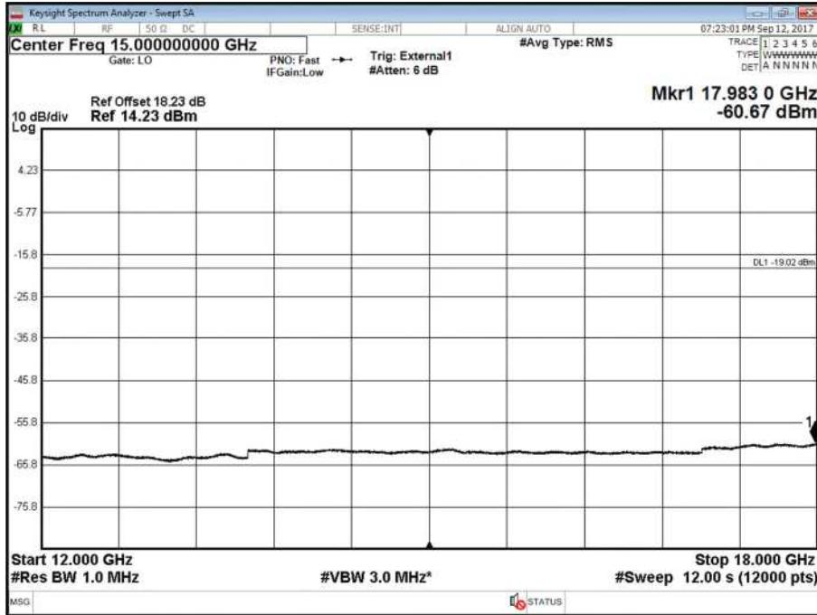
Antenna B - LTE Modulation QPSK - LTE Carrier Bandwidth 10.0 MHz - Channel Position T - Band 4 - Range 18000 to 27000 MHz
