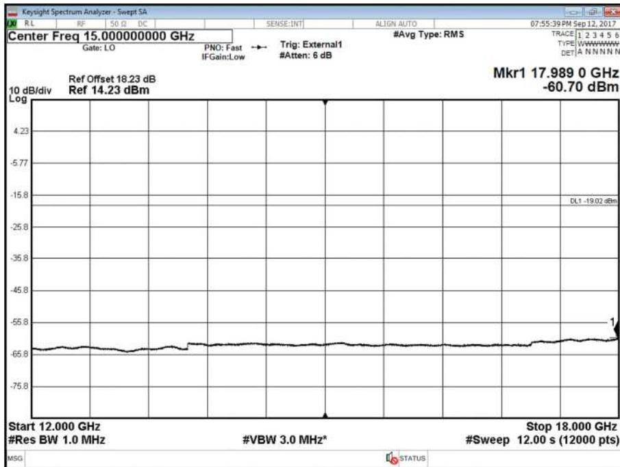
Antenna B - LTE Modulation QPSK - LTE Carrier Bandwidth 15.0 MHz - Channel Position T - Band 4 - Range 18000 to 27000 MHz
