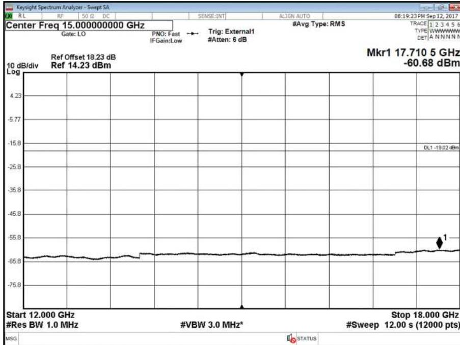
Antenna B - LTE Modulation QPSK - LTE Carrier Bandwidth 20.0 MHz - Channel Position M - Band 4 - Range 18000 to 27000 MHz
