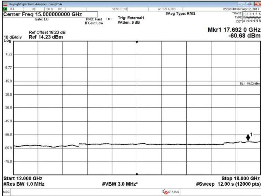
Antenna A - LTE Modulation QPSK - LTE Carrier Bandwidth 15.0 MHz - Channel Position B - Band 4 - Range 18000 to 27000 MHz
