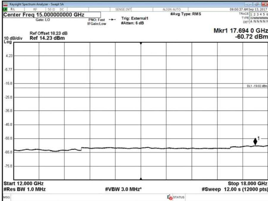
Antenna B - LTE Modulation QPSK - LTE Carrier Bandwidth 5.0 MHz - Channel Position T - Band 4 - Range 18000 to 27000 MHz
