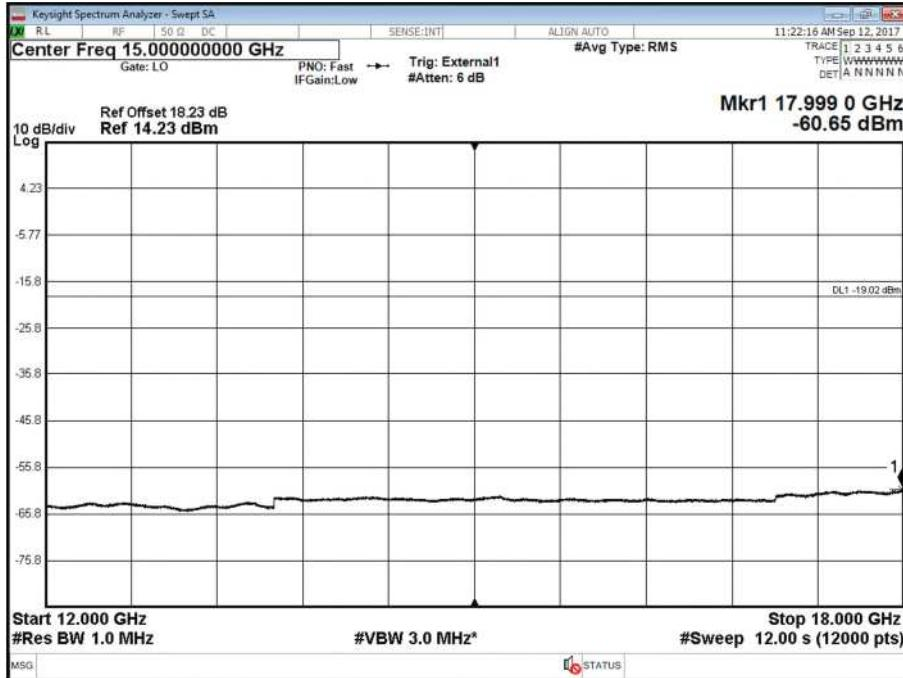
Antenna A - LTE Modulation QPSK - LTE Carrier Bandwidth 5.0 MHz - Channel Position M - Band 4 - Range 18000 to 27000 MHz
