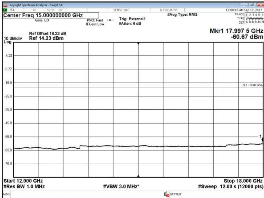
Antenna A - LTE Modulation QPSK - LTE Carrier Bandwidth 5.0 MHz - Channel Position B - Band 4 - Range 18000 to 27000 MHz
