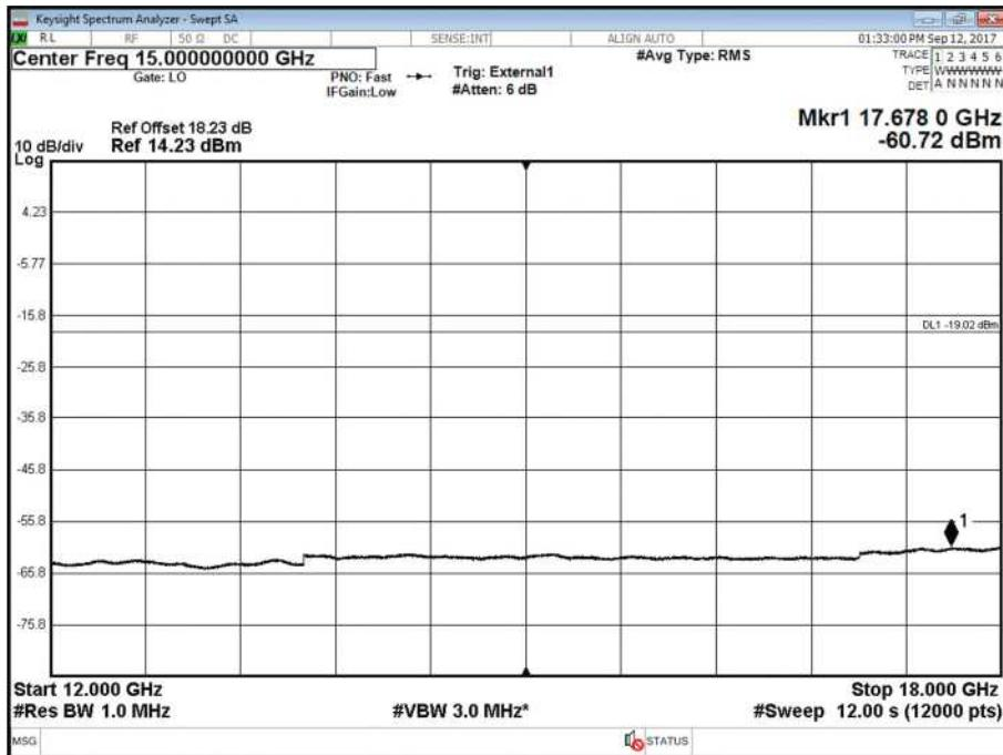
Antenna A - LTE Modulation QPSK - LTE Carrier Bandwidth 10.0 MHz - Channel Position T - Band 4 - Range 18000 to 27000 MHz
