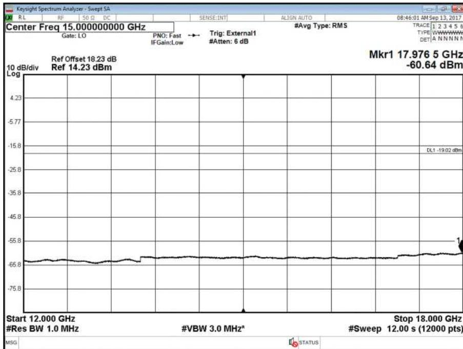
Antenna B - LTE Modulation QPSK - LTE Carrier Bandwidth 5.0 MHz - Channel Position M - Band 4 - Range 18000 to 27000 MHz
