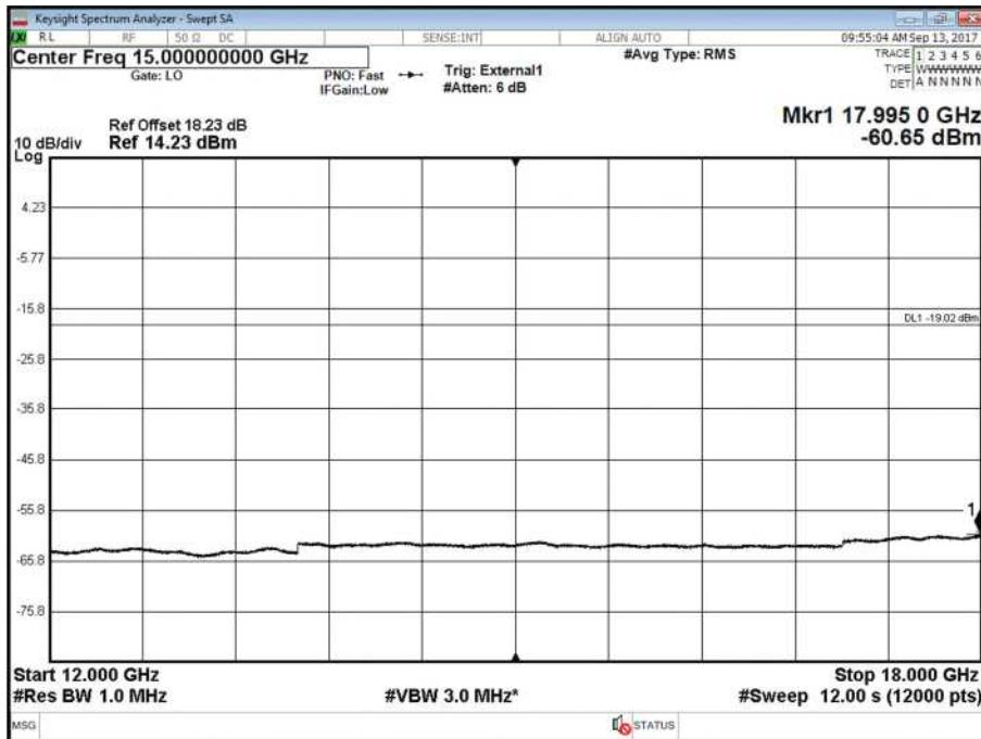
Antenna B - LTE Modulation QPSK - LTE Carrier Bandwidth 15.0 MHz - Channel Position M - Band 4 - Range 18000 to 27000 MHz
