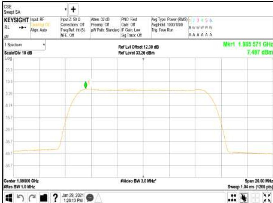
Antenna Port A Carrier Power - Modulation LTE: QPSK - Carrier Bandwidth 15.0 MHz - Channel Position T
