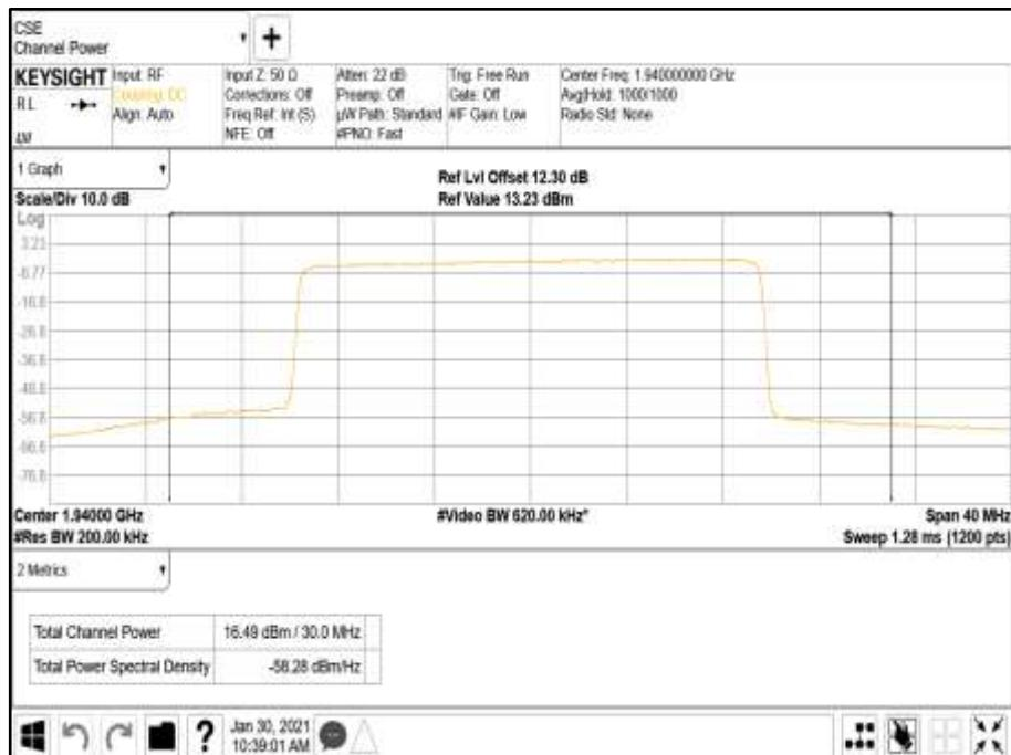
Antenna Port A Pk-Av Ratio - Modulation NR: QPSK - Carrier Bandwidth 20.0 MHz - Channel Position B
