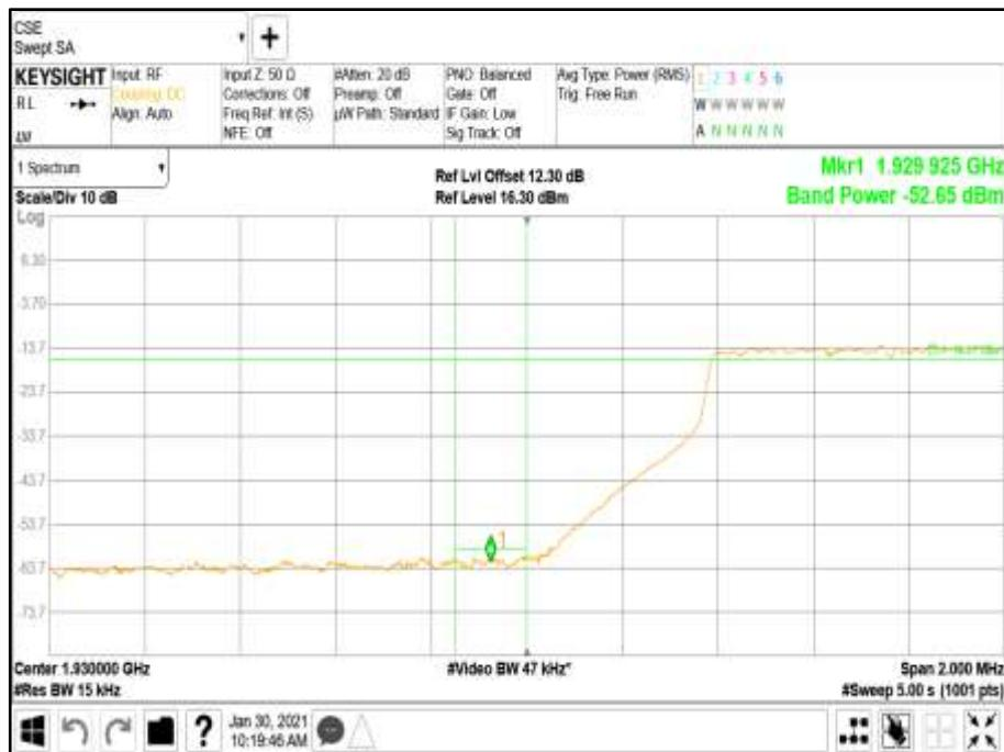
Modulation NR: QPSK - Carrier Bandwidth NR: 15.0 MHz - Channel Position T
