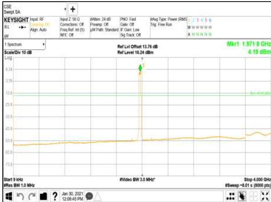
Modulation LTE+NR: QPSK - Carrier Bandwidth 5.0 MHz - Channel Position M - Band 2.00 - Range 4000 to 12000 MHz
