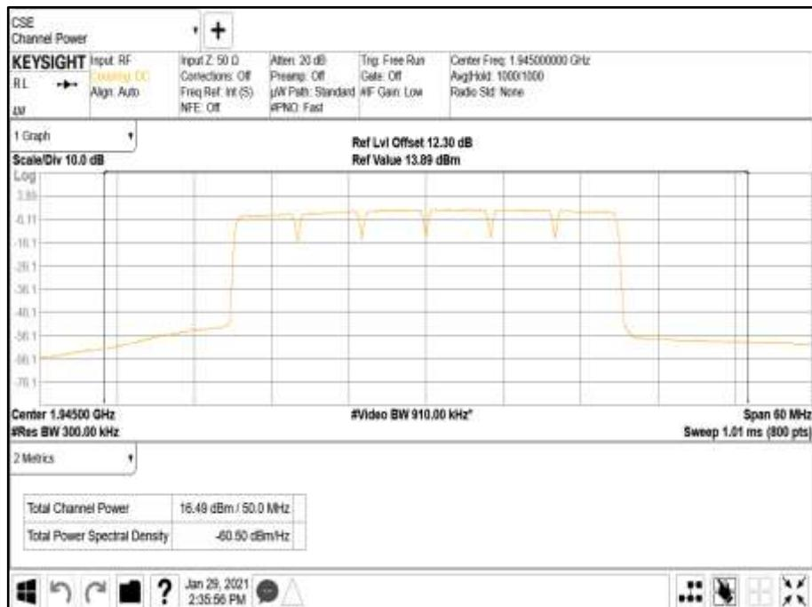
Antenna A - Modulation NR: QPSK - Carrier Bandwidth 5.0+5.0+5.0+5.0+5.0+5.0 MHz - Channel Position B
