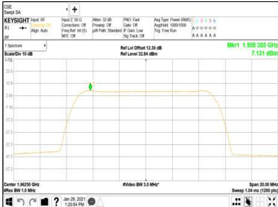
Antenna Port A Carrier Power - Modulation LTE: QPSK - Carrier Bandwidth 15.0 MHz - Channel Position M
