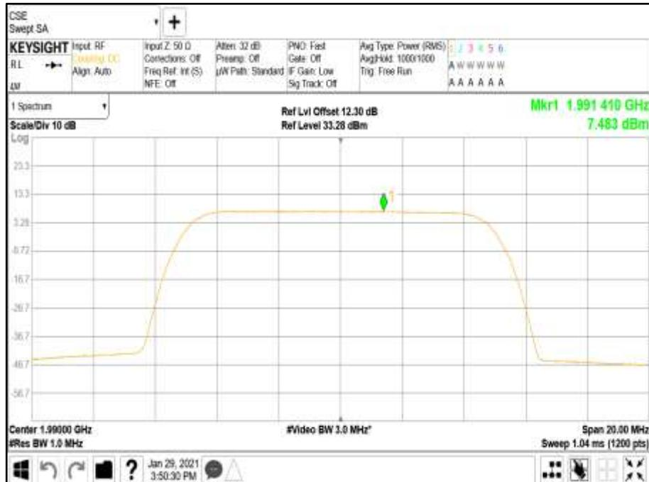
Antenna Port A Carrier Power - Modulation NR: QPSK - Carrier Bandwidth 15.0 MHz - Channel Position T
