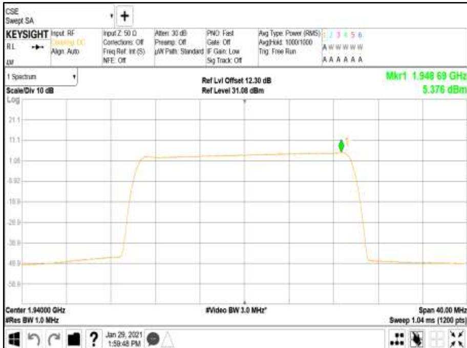
Antenna Port A Carrier Power - Modulation NR: QPSK - Carrier Bandwidth 5.0 MHz - Channel Position B
