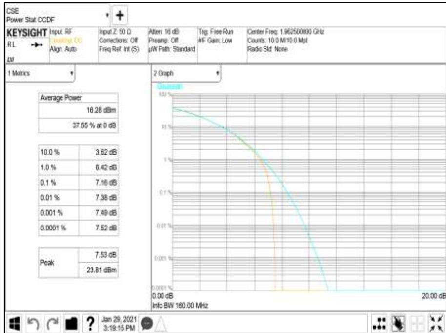
Antenna Port A PSD - Modulation NR: QPSK - Carrier Bandwidth 5.0 MHz - Channel Position M
