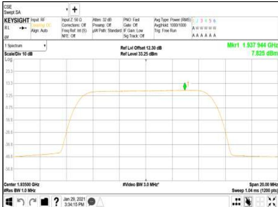
Antenna Port A Carrier Power - Modulation NR: QPSK - Carrier Bandwidth 15.0 MHz - Channel Position B
