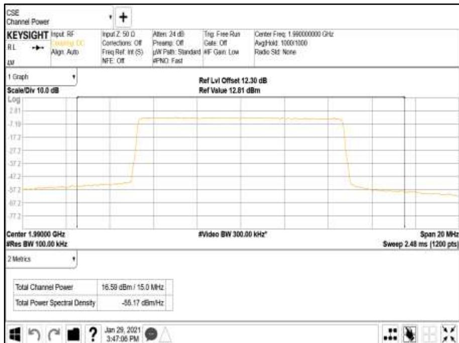
Antenna Port A Pk-Av Ratio - Modulation NR: QPSK - Carrier Bandwidth 10.0 MHz - Channel Position T
