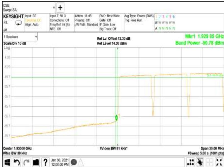
Antenna A - Modulation LTE + NR QPSK - Carrier Bandwidth 5.0+5.0+5.0+5.0+5.0+5.0 MHz - Channel Position T
