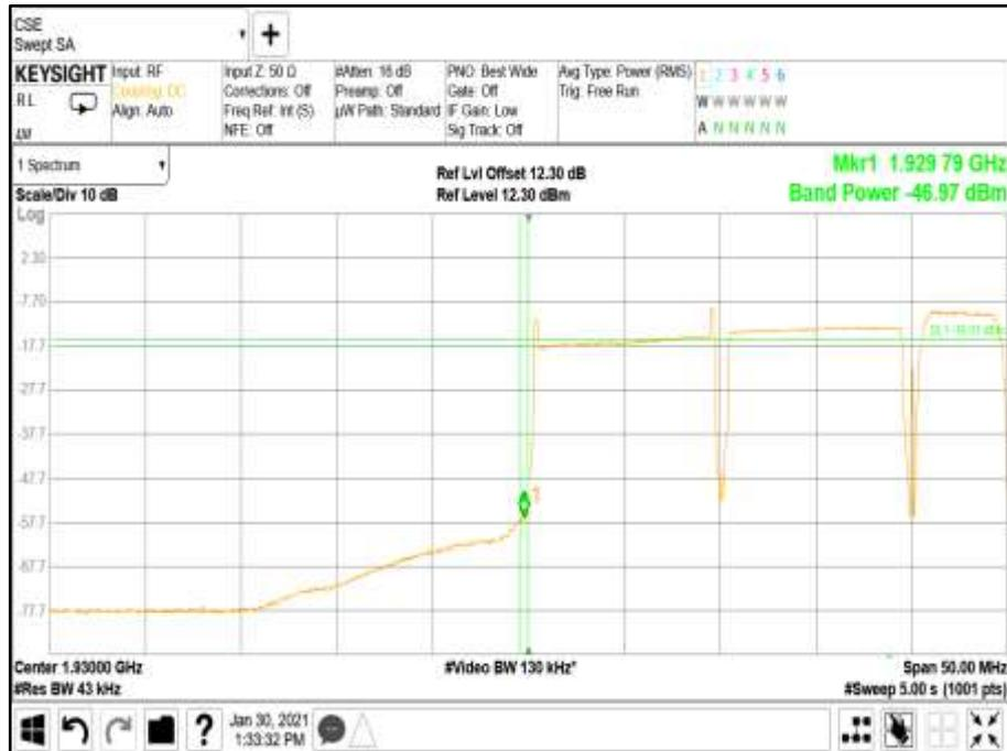
Antenna A - Modulation LTE + WCDMA QPSK - Carrier Bandwidth 10.0+10.0+5.0+5.0+5.0+5.0 MHz - Channel Position T
