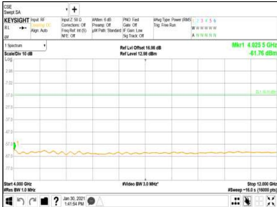
Modulation LTE+WCDMA: QPSK - Carrier Bandwidth 5.0 MHz - Channel Position M - Band 3.00 - Range 12000 to 20000 MHz
