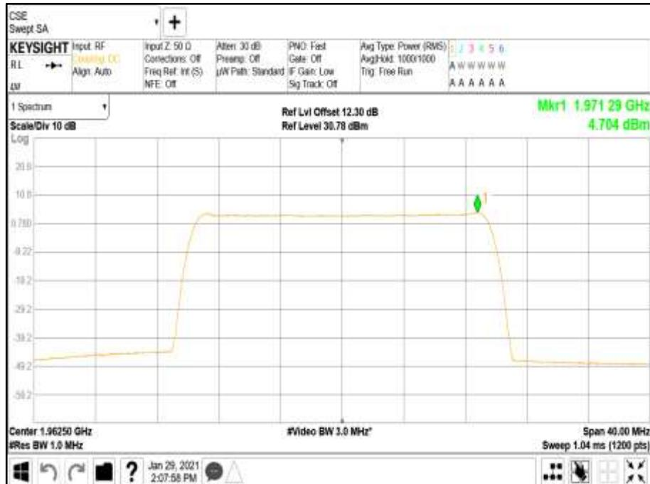
Antenna Port A Carrier Power - Modulation NR: QPSK - Carrier Bandwidth 5.0 MHz - Channel Position M
