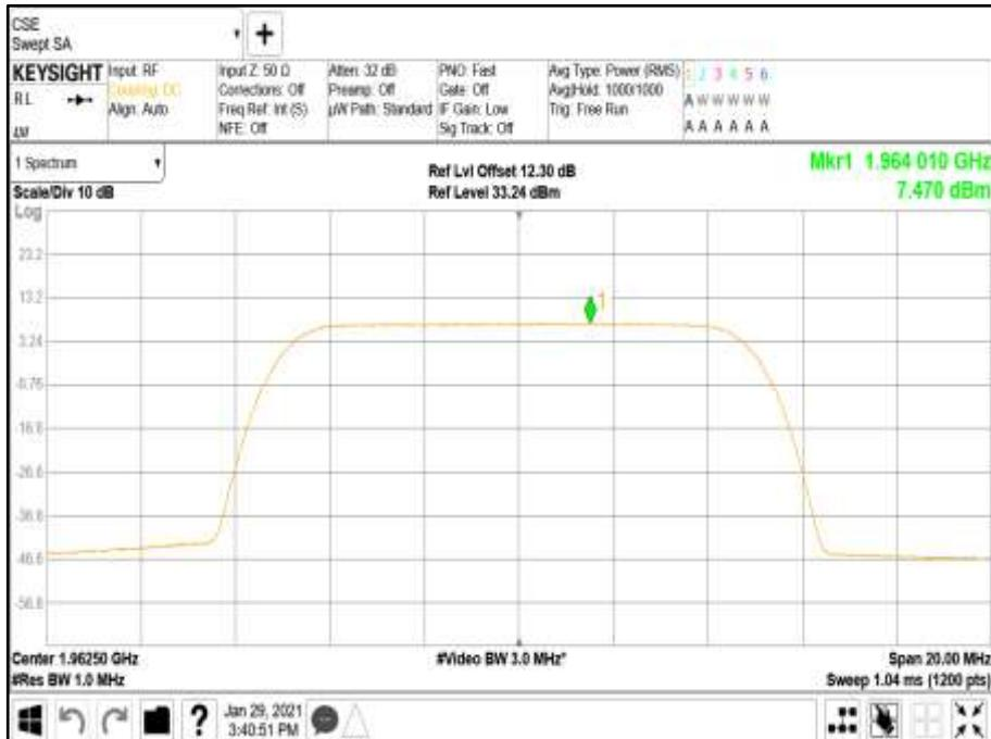
Antenna Port A Carrier Power - Modulation NR: QPSK - Carrier Bandwidth 15.0 MHz - Channel Position M
