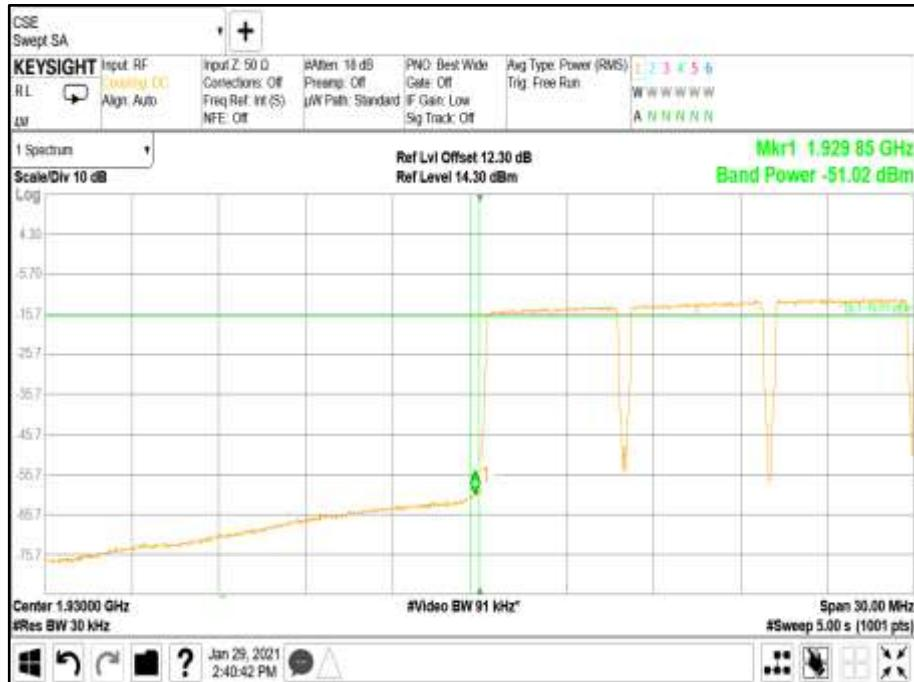
Antenna A - Modulation LTE: QPSK - Carrier Bandwidth 5.0+5.0+5.0+5.0+5.0+5.0 MHz - Channel Position T
