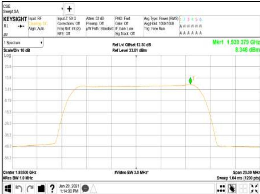
Antenna Port A Carrier Power - Modulation LTE: QPSK - Carrier Bandwidth 15.0 MHz - Channel Position B
