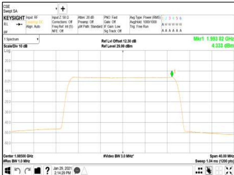
Antenna Port A Carrier Power - Modulation NR: QPSK - Carrier Bandwidth 5.0 MHz - Channel Position T
