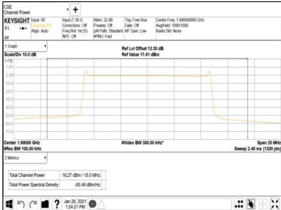
Antenna Port A Pk-Av Ratio - Modulation LTE: QPSK - Carrier Bandwidth 10.0 MHz - Channel Position T
