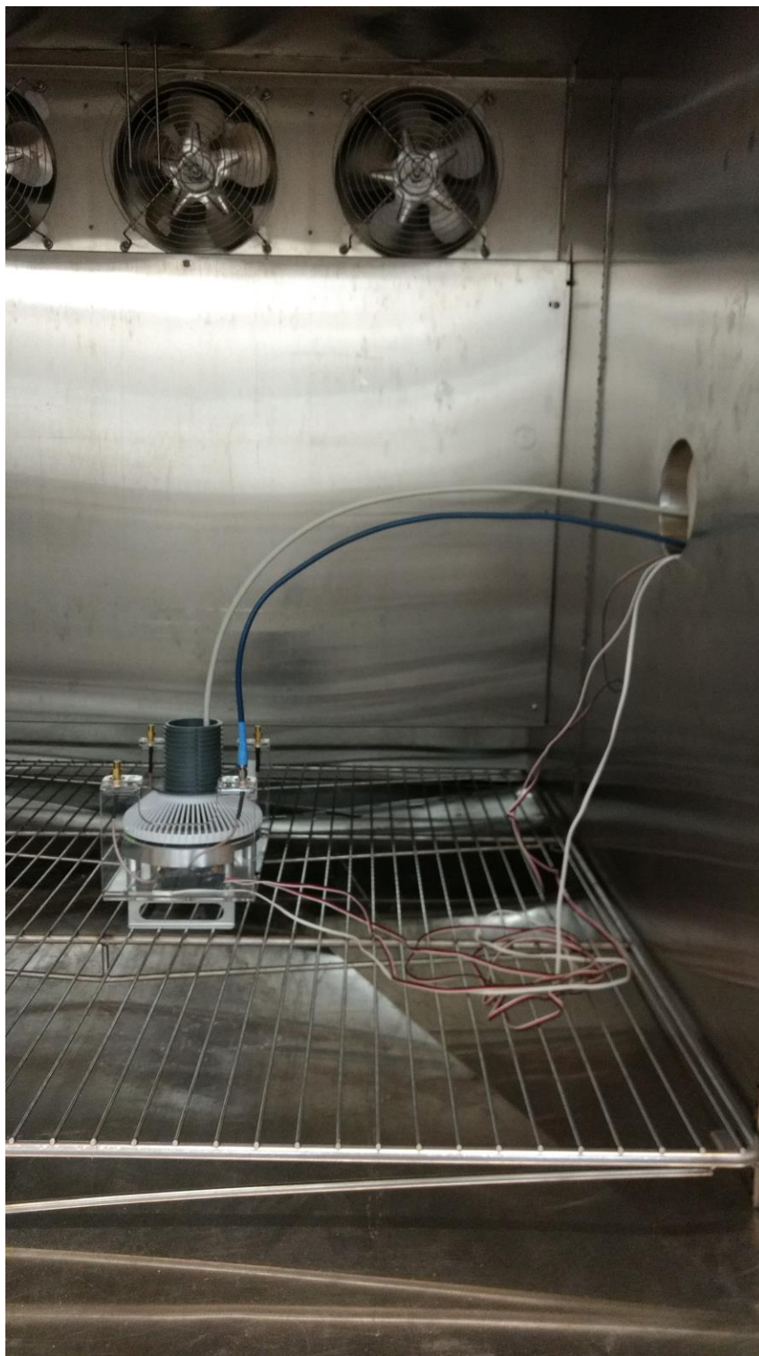
Figure 4: EUT test fixture in a thermal test chamber
