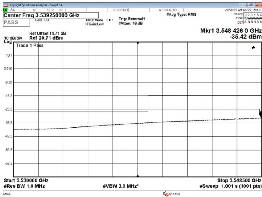
Antenna C - LTE Modulation QPSK - LTE Carrier Bandwidth 5.0 MHz - Channel Position B -
