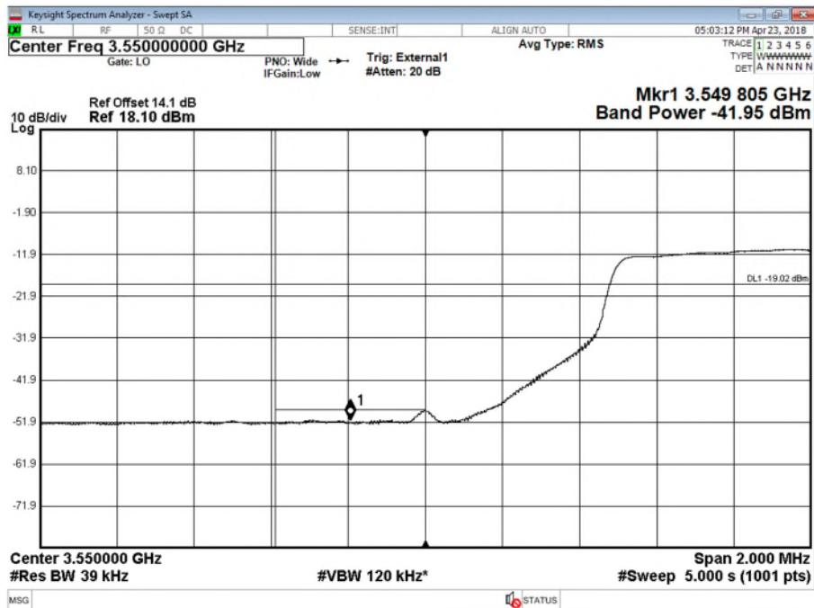
Antenna B - LTE Modulation QPSK - LTE Carrier Bandwidth 10.0 MHz - Channel Position B
