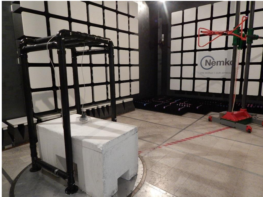
Figure 7.1-21: Radiated emissions setup photo
