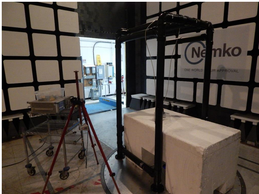
Figure 7.1-24: Radiated emissions setup photo
