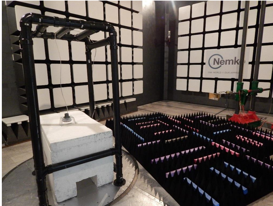
Figure 7.1-23: Radiated emissions setup photo
