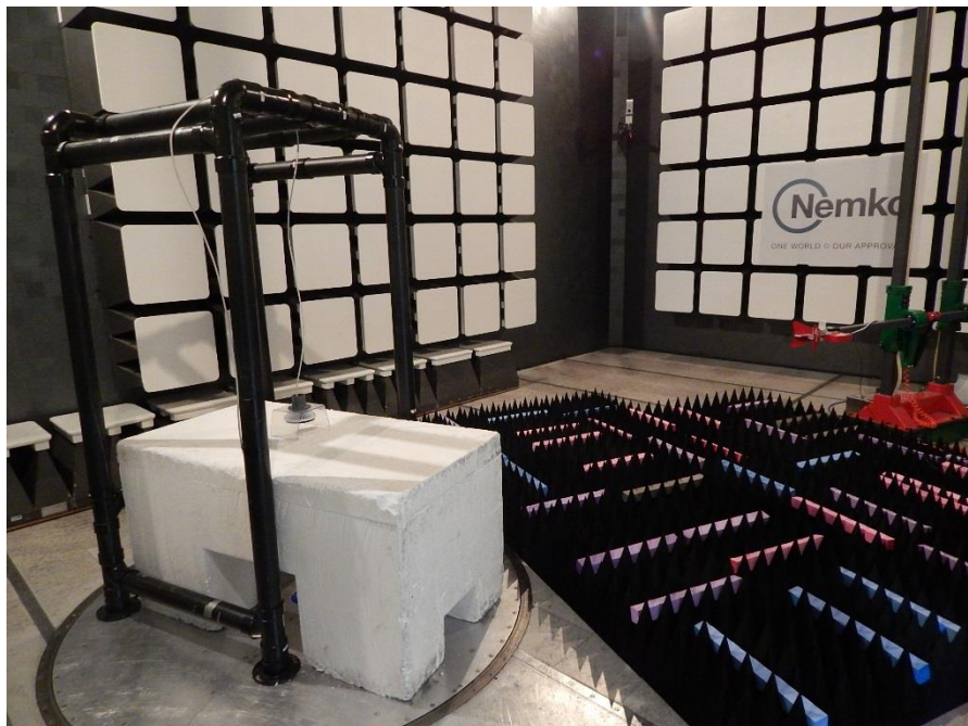
Figure 7.1-22: Radiated emissions setup photo
