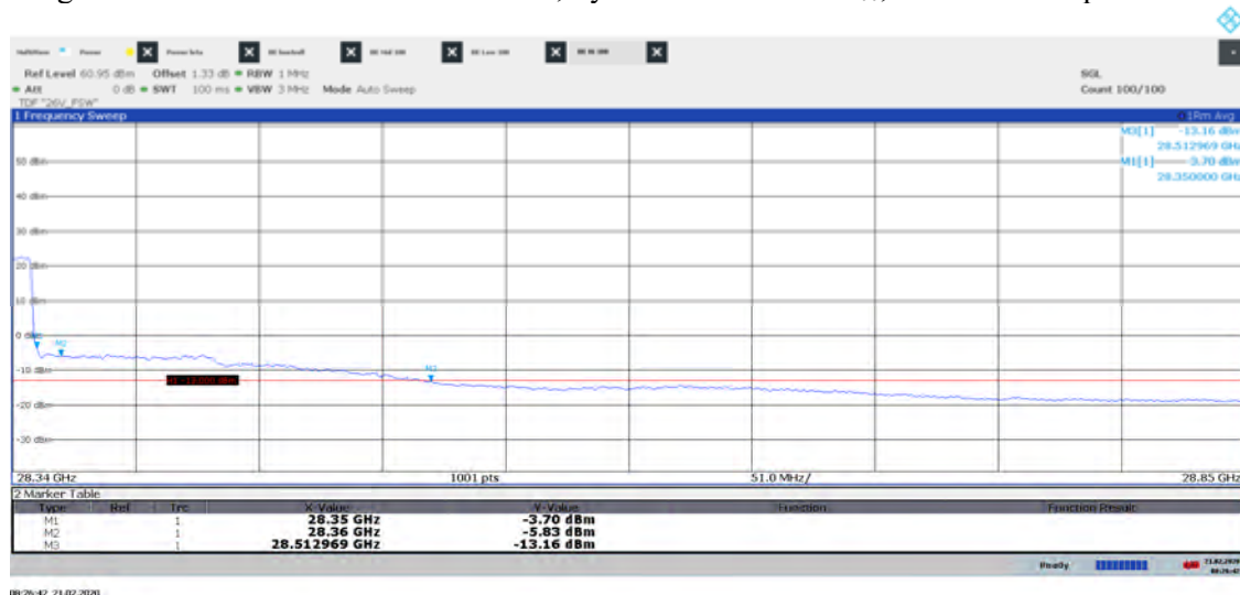
Diagram 24f: Pre scan 28.34 – 28.85 GHz, Symbolic name: BT8 100 , EIRP Vertical polarization
