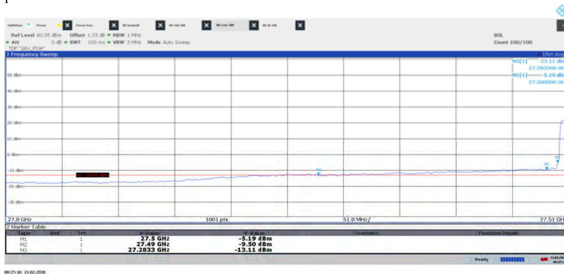
Diagram 24d: Pre scan 27.00 – 27.51 GHz, Symbolic name: BT8 100 , EIRP Vertical polarization
