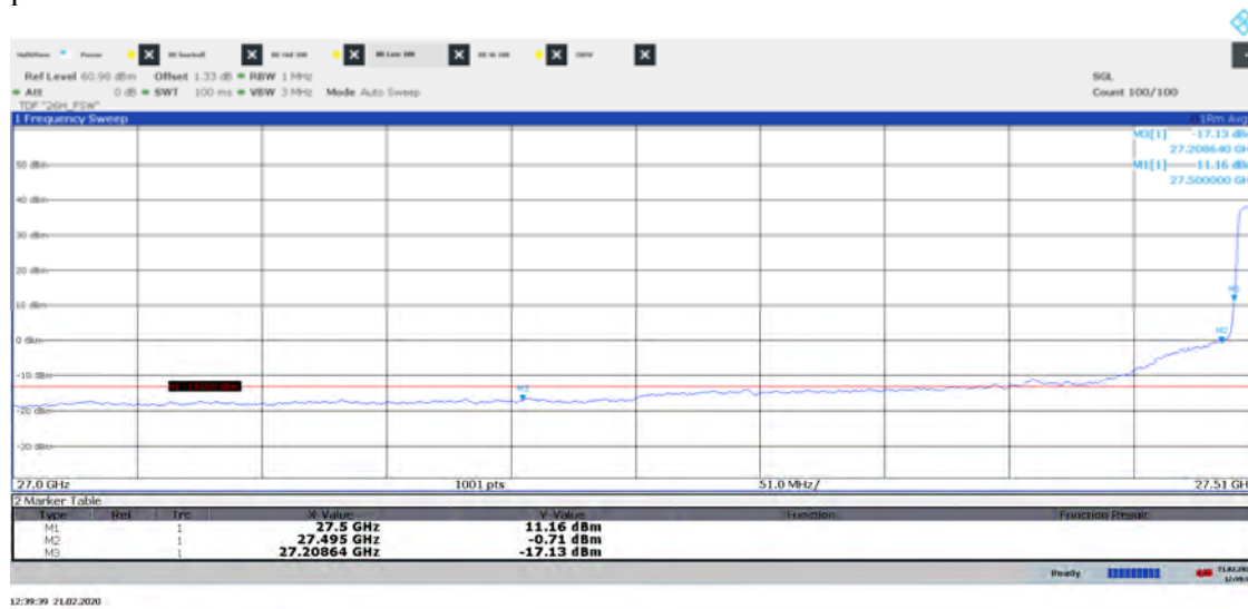
Diagram 17c: Pre scan 27.00 – 27.51 GHz, Symbolic name: BL 100 , EIRP Horizontal polarization
