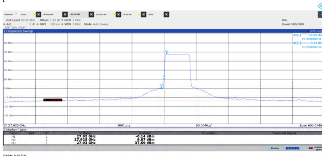
Diagram 20b: Pre scan 27.625 – 28.225 GHz, Symbolic name: BH 50 , EIRP Vertical polarization
