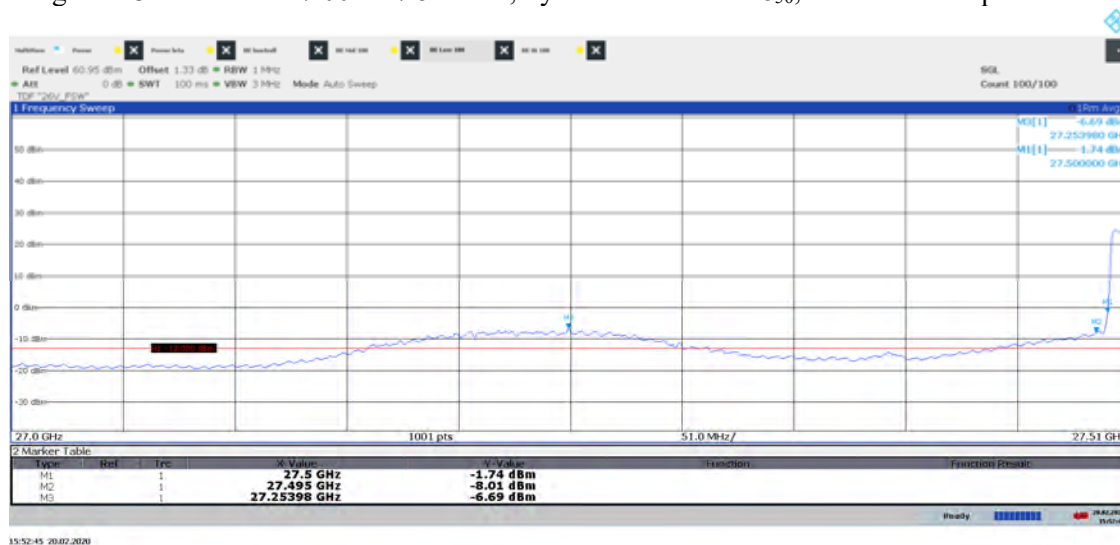
Diagram 23d: Pre scan 27.00 – 27.51 GHz, Symbolic name: BT8 50 , EIRP Vertical polarization
