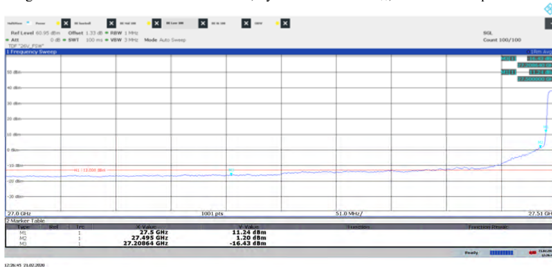
Diagram 17d: Pre scan 27.00 – 27.51 GHz, Symbolic name: BL 100 , EIRP Vertical polarization
