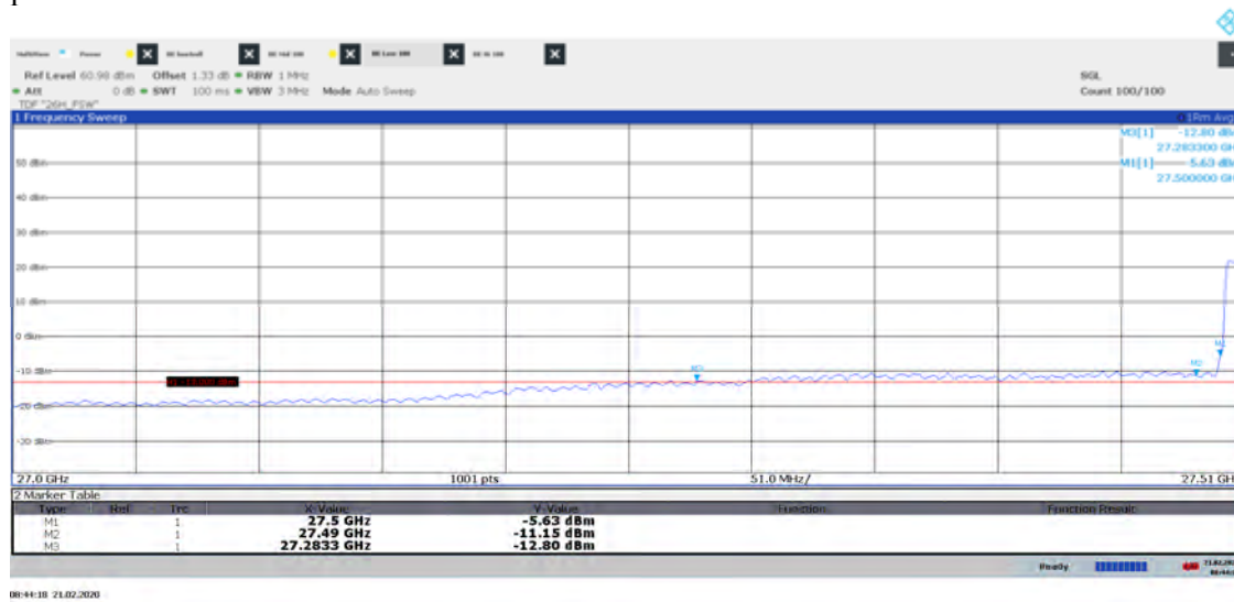
Diagram 24c: Pre scan 27.00 – 27.51 GHz, Symbolic name: BT8 100 EIRP Horizontal polarization
