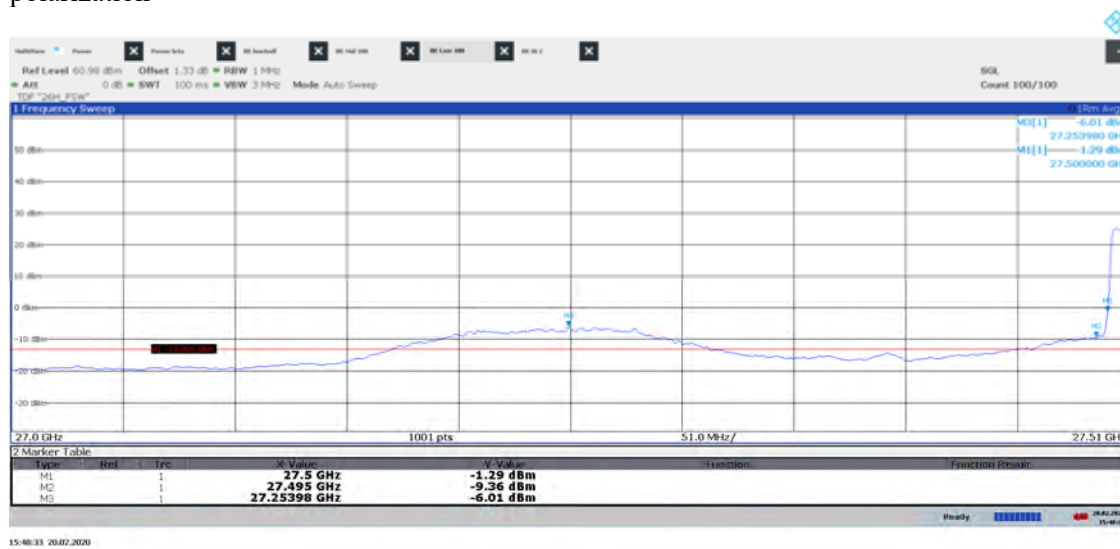
Diagram 23c: Pre scan 27.00 – 27.51 GHz, Symbolic name: BT8 50 , EIRP Horizontal polarization
