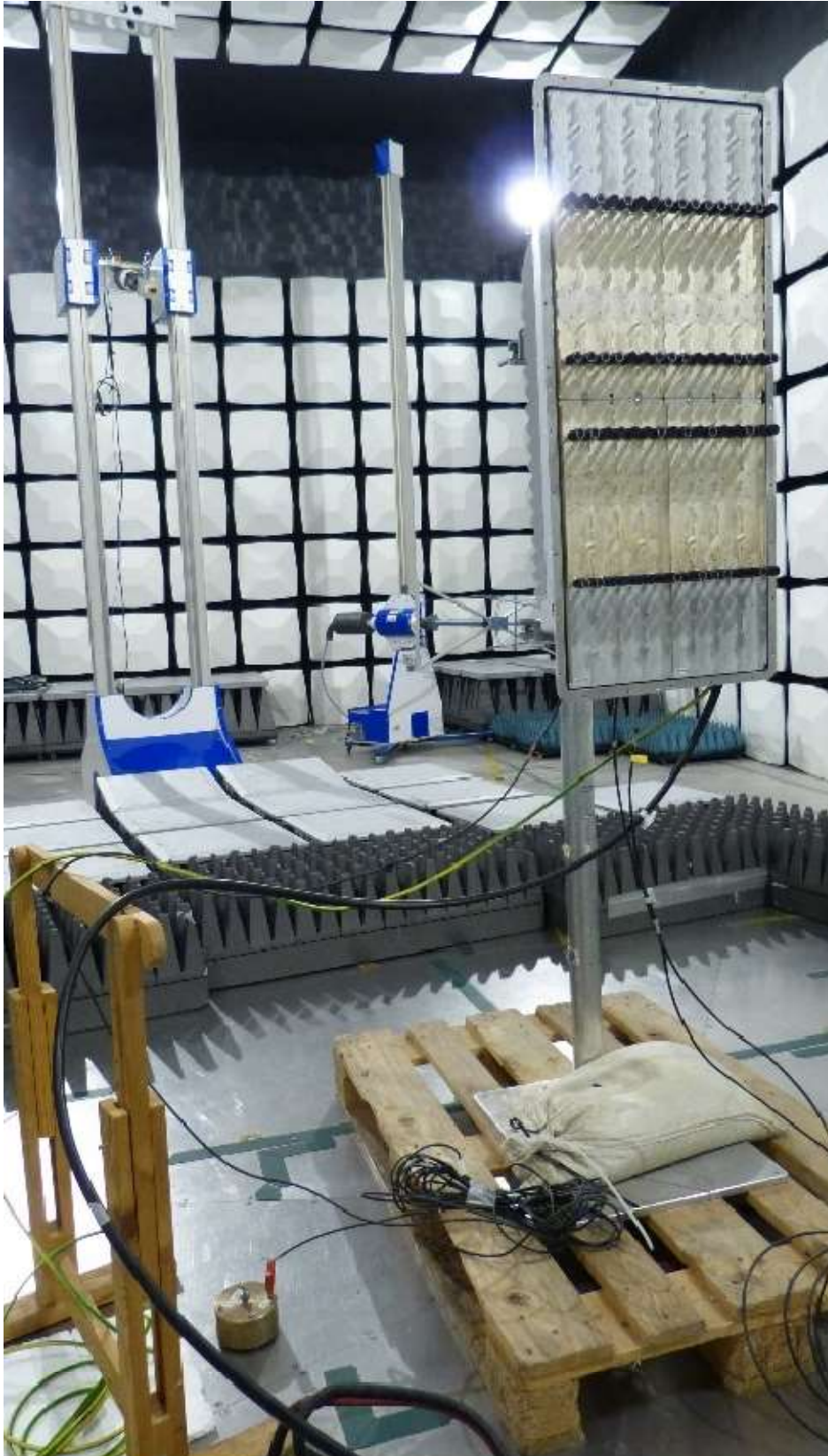
Photo of the test set-up for radiated emission above 26,5 – 40 GHz
