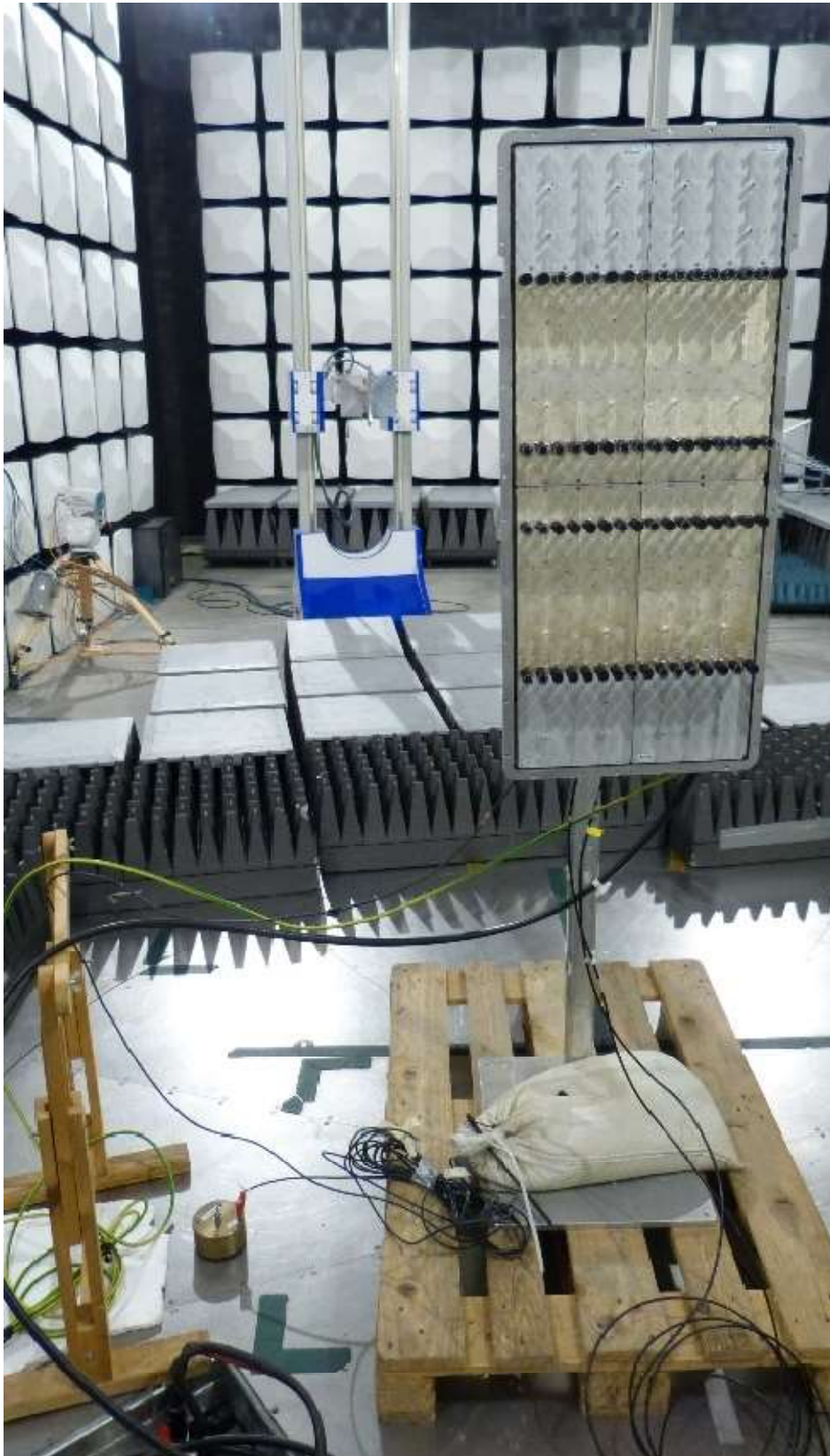
Photo of the test set-up for radiated emission above 1 – 18 GHz
