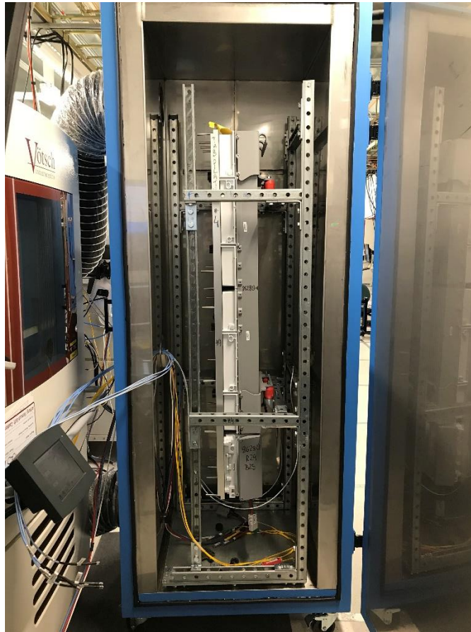
Figure 3.6-2: EUT Set-up for Radio Compliance Testing
