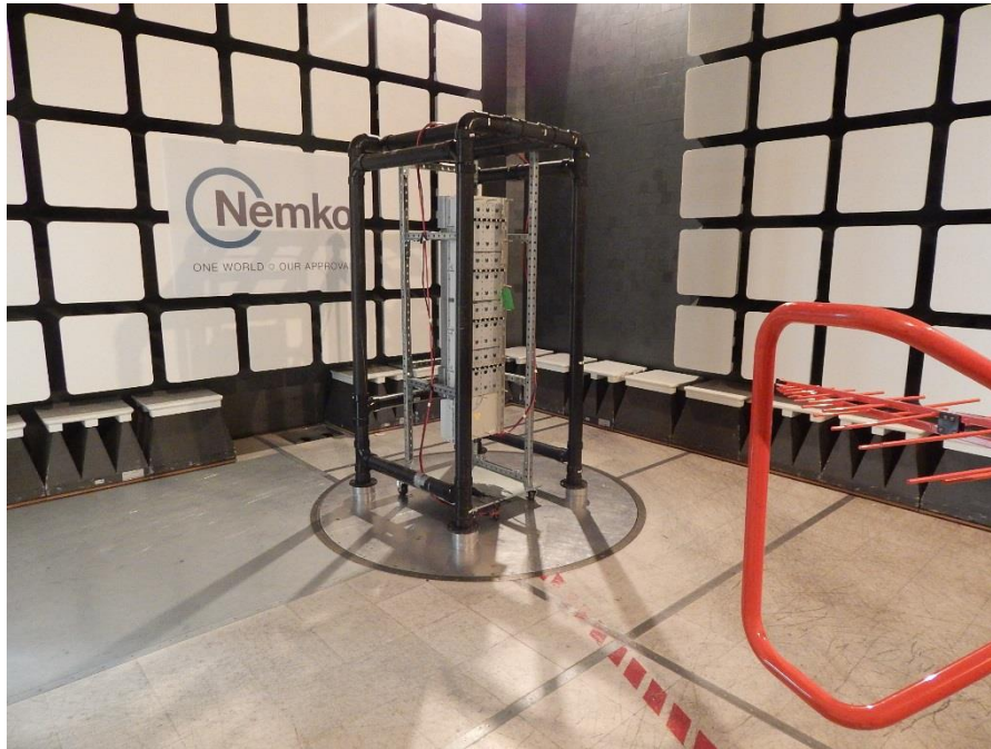
Figure 8.3-1: Radiated emissions setup photo – below 1 GHz
