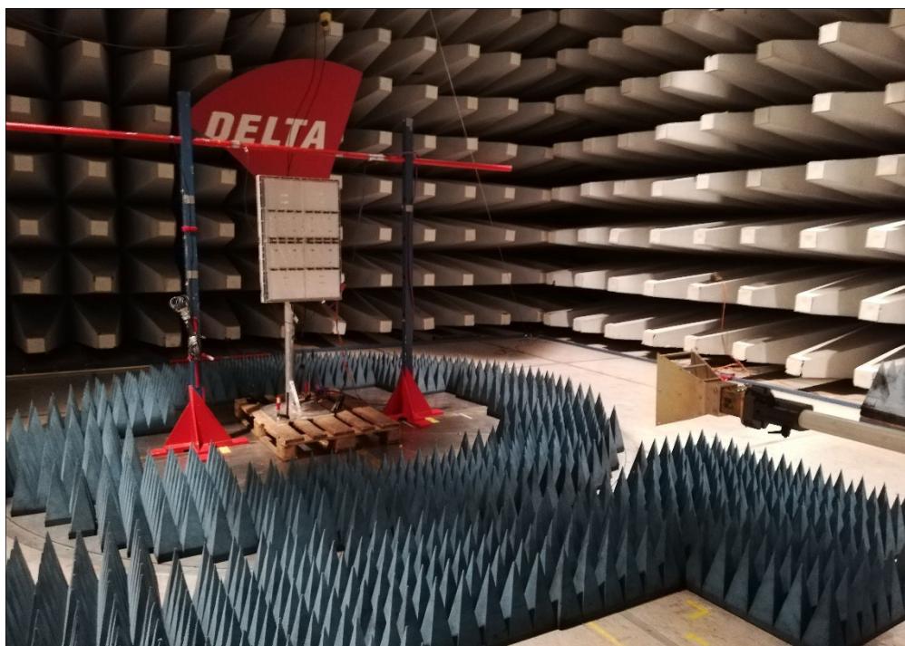
Figure 20 - Test Setup - 1 GHz to 18 GHz
