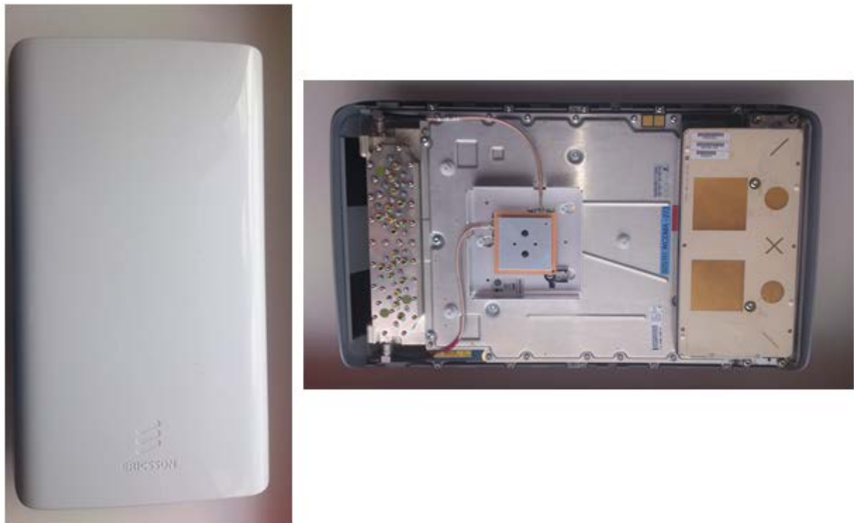
Figure A.1 Front view of the EUT and EUT with radome removed showing the WCDMA and WiFi antennas.
