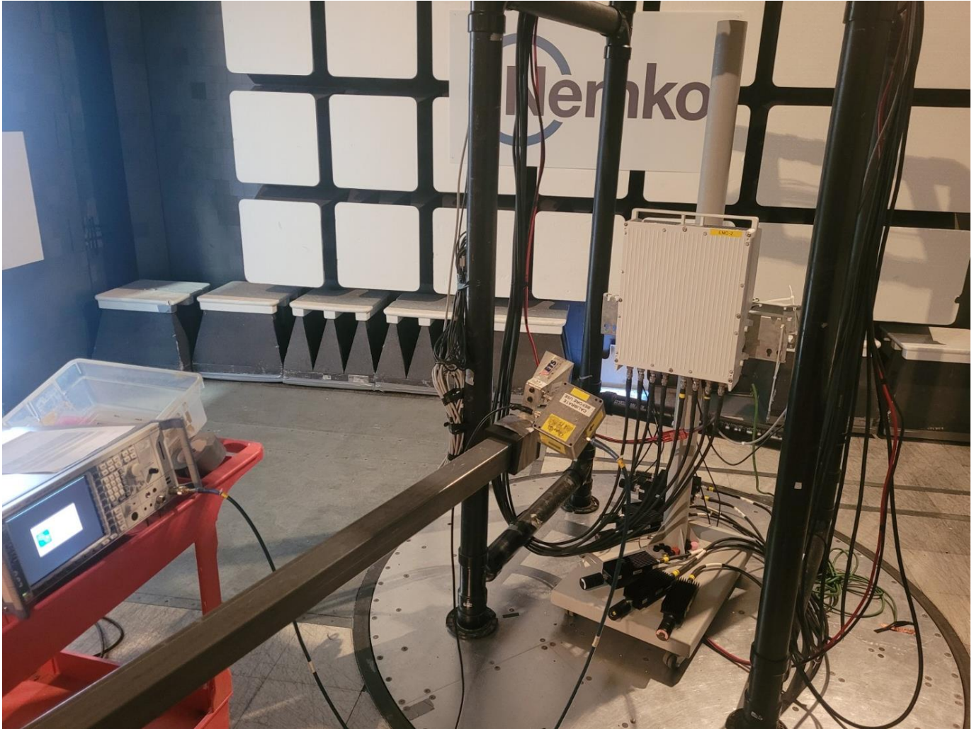
Figure 3.5-6: EUT Set-up photo for Radiated Emissions [18-40 GHz]
