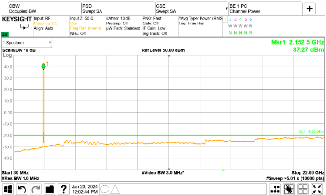
Figure 8.3-26: Conducted spurious emissions of NR 5 MHz, WCDMA and LTE 5 MHz, noncontiguous, 3 carrier operation
