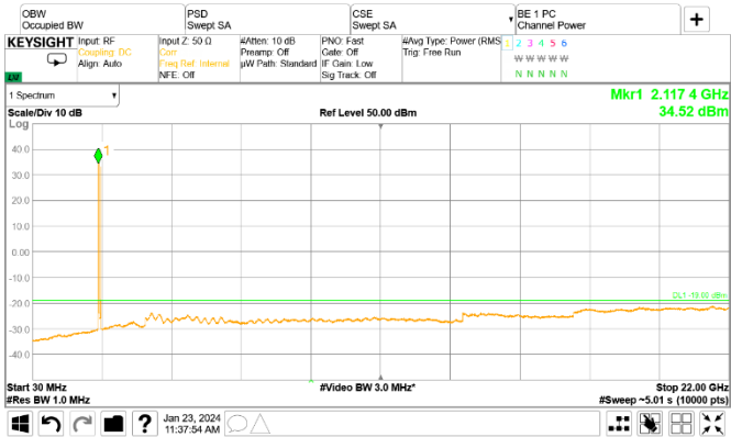
Figure 8.3-25: Conducted spurious emissions of WCDMA, NR 5 MHz and LTE 5 MHz, noncontiguous, 6 carrier operation
