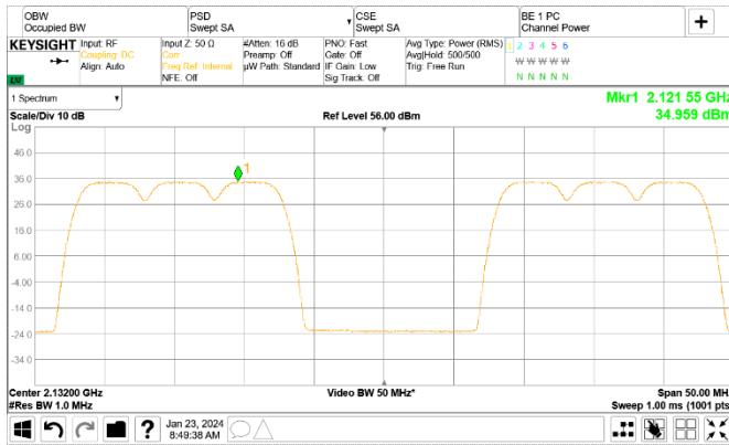
Figure 8.1-7: PSD of WCDMA, 6 carrier noncontiguous operation
