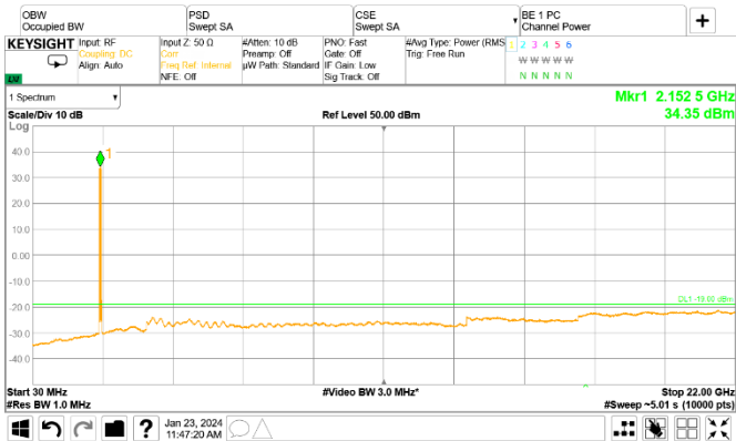
Figure 8.3-27: Conducted spurious emissions of NR 5 MHz, WCDMA and LTE 5 MHz, noncontiguous, 6 carrier operation
