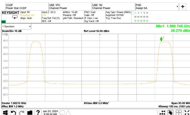
Figure 8.2-9: PSD of WCDMA and LTE, 2 carrier noncontiguous operation
