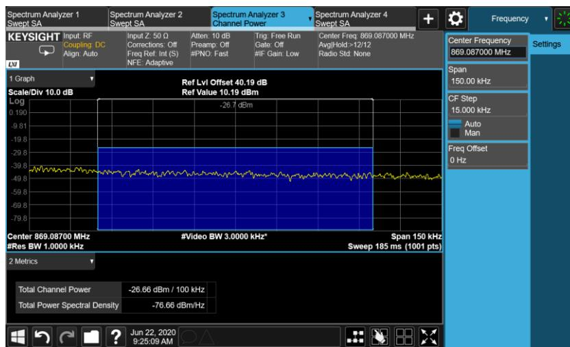
The channel power of 100KHz for 869.087MHz is -26.66dBm, which is within the limit of -19.02dBm.
