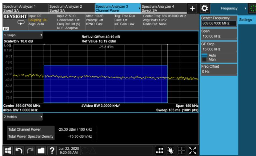
The channel power of 100KHz for 869.087MHz is -25.30dBm, which is within the limit of -19.02dBm.
