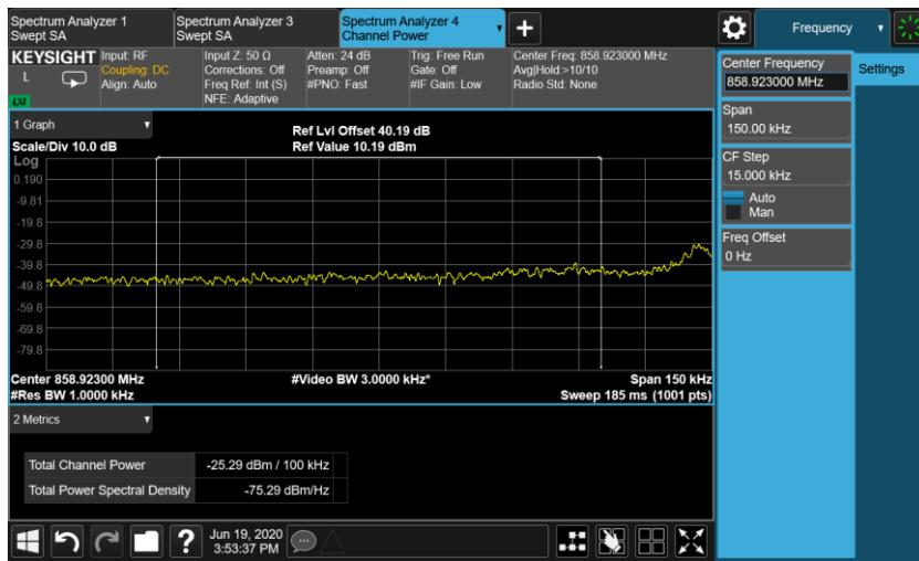
The channel power of 100KHz for 858.923MHz is -25.29dBm, which is within the limit of -19.02dBm.
