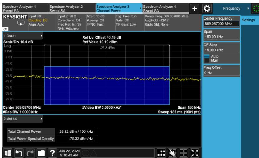
The channel power of 100KHz for 869.087MHz is -25.32dBm, which is within the limit of -19.02dBm.
