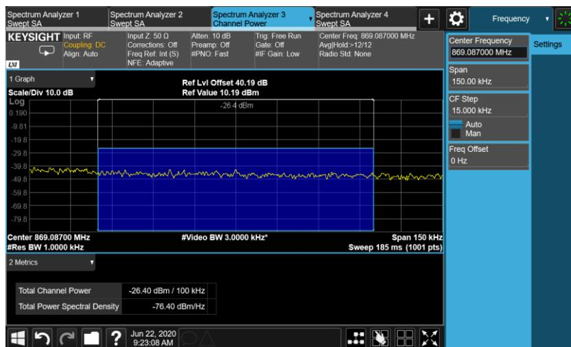
The channel power of 100KHz for 869.087MHz is -26.40dBm, which is within the limit of -19.02dBm.
