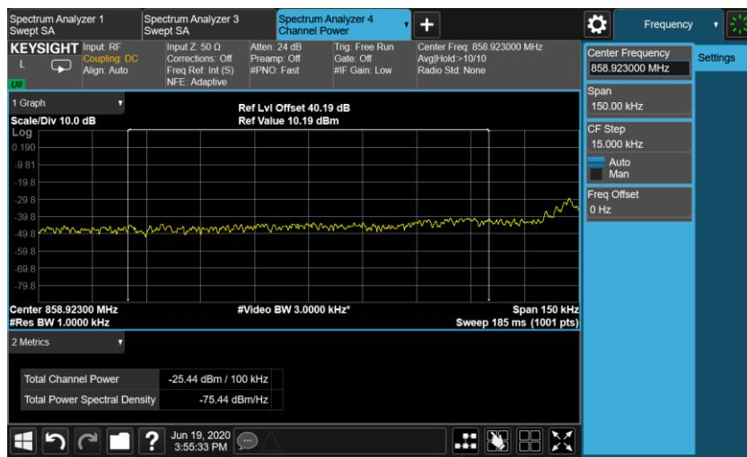
The channel power of 100KHz for 858.923MHz is -25.44dBm, which is within the limit of -19.02dBm.
