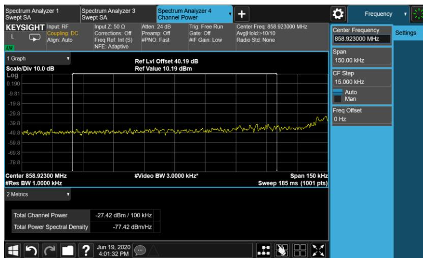
The channel power of 100KHz for 858.923MHz is -27.42dBm, which is within the limit of -19.02dBm.
