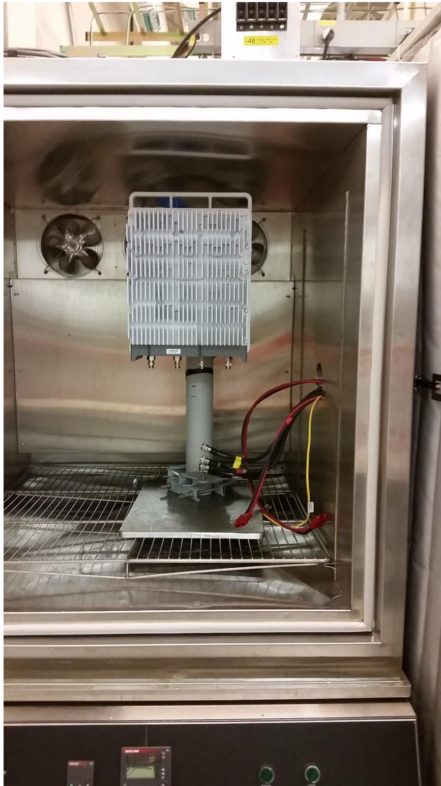
Figure 3.6-2: EUT Set-up for Radio Compliance Testing
