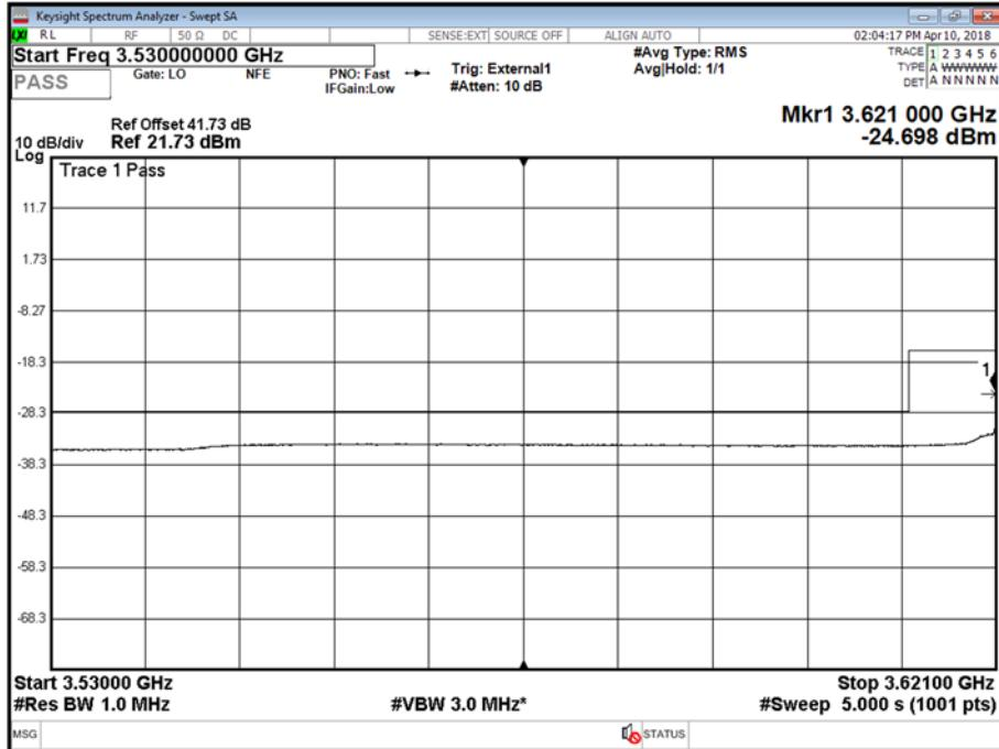
Antenna A - LTE Modulation 64QAM - LTE Carrier Bandwidth 5.0 MHz - Channel Position M - Band edge - Range edge low
