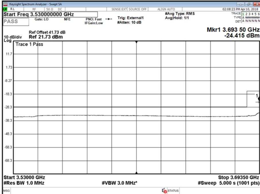
Antenna A - LTE Modulation 64QAM - LTE Carrier Bandwidth 5.0 MHz - Channel Position T - Band edge - Range edge low
