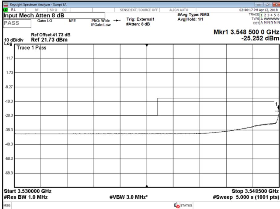
Antenna B - LTE Modulation 64QAM - LTE Carrier Bandwidth 5.0 MHz - Channel Position B - Band edge - Range edge low
