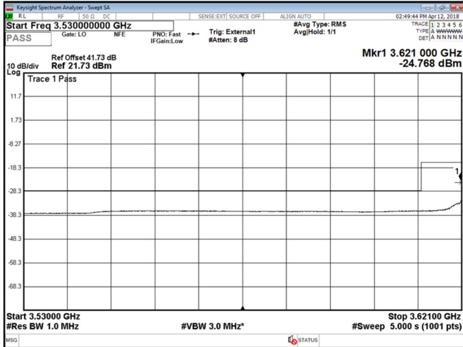
Antenna B - LTE Modulation 64QAM - LTE Carrier Bandwidth 5.0 MHz - Channel Position M - Band edge - Range edge low
