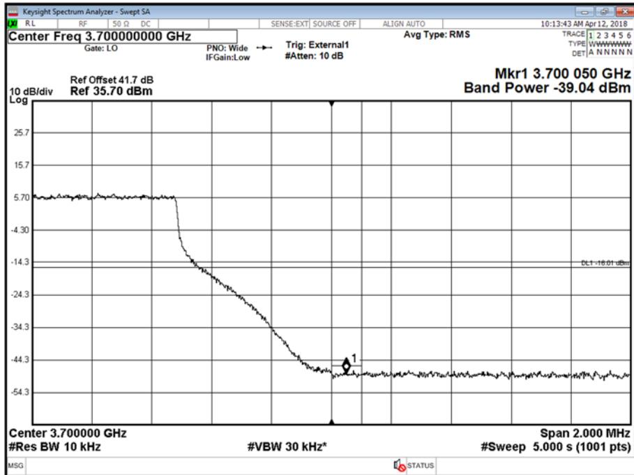
Antenna A - LTE Modulation 64QAM - LTE Carrier Bandwidth 20.0 MHz - Channel Position B
