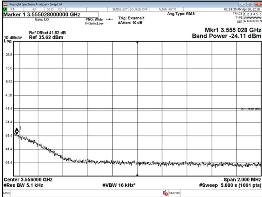
Antenna A - LTE Modulation 64QAM - LTE Carrier Bandwidth 5.0 MHz - Channel Position B - Band mask high - Range High
