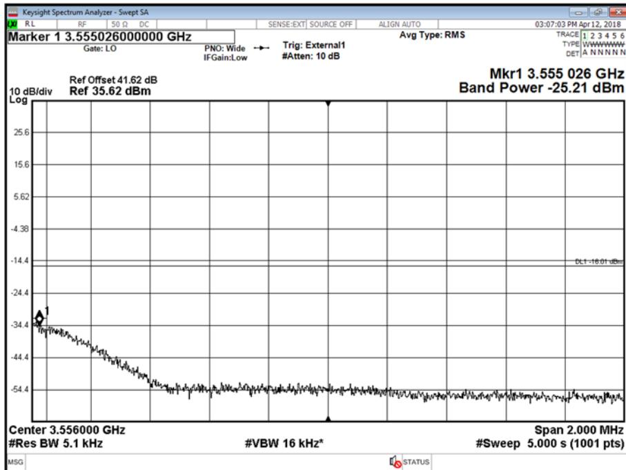
Antenna B - LTE Modulation 64QAM - LTE Carrier Bandwidth 5.0 MHz - Channel Position B - Band mask high - Range High
