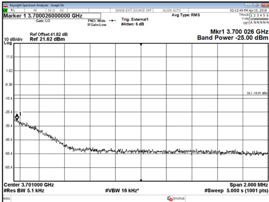
Antenna A - LTE Modulation 64QAM - LTE Carrier Bandwidth 5.0 MHz - Channel Position T - Band mask high - Range High
