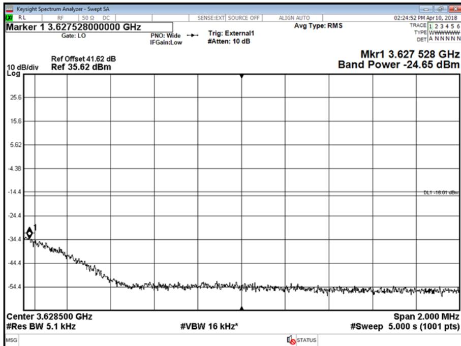
Antenna A - LTE Modulation 64QAM - LTE Carrier Bandwidth 5.0 MHz - Channel Position M - Band mask high - Range High
