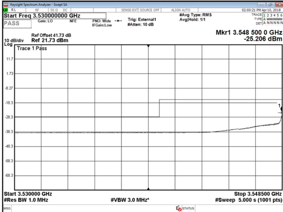
Antenna A - LTE Modulation 64QAM - LTE Carrier Bandwidth 5.0 MHz - Channel Position B - Band edge - Range edge low
