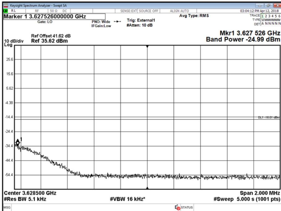
Antenna B - LTE Modulation 64QAM - LTE Carrier Bandwidth 5.0 MHz - Channel Position M - Band mask high - Range High
