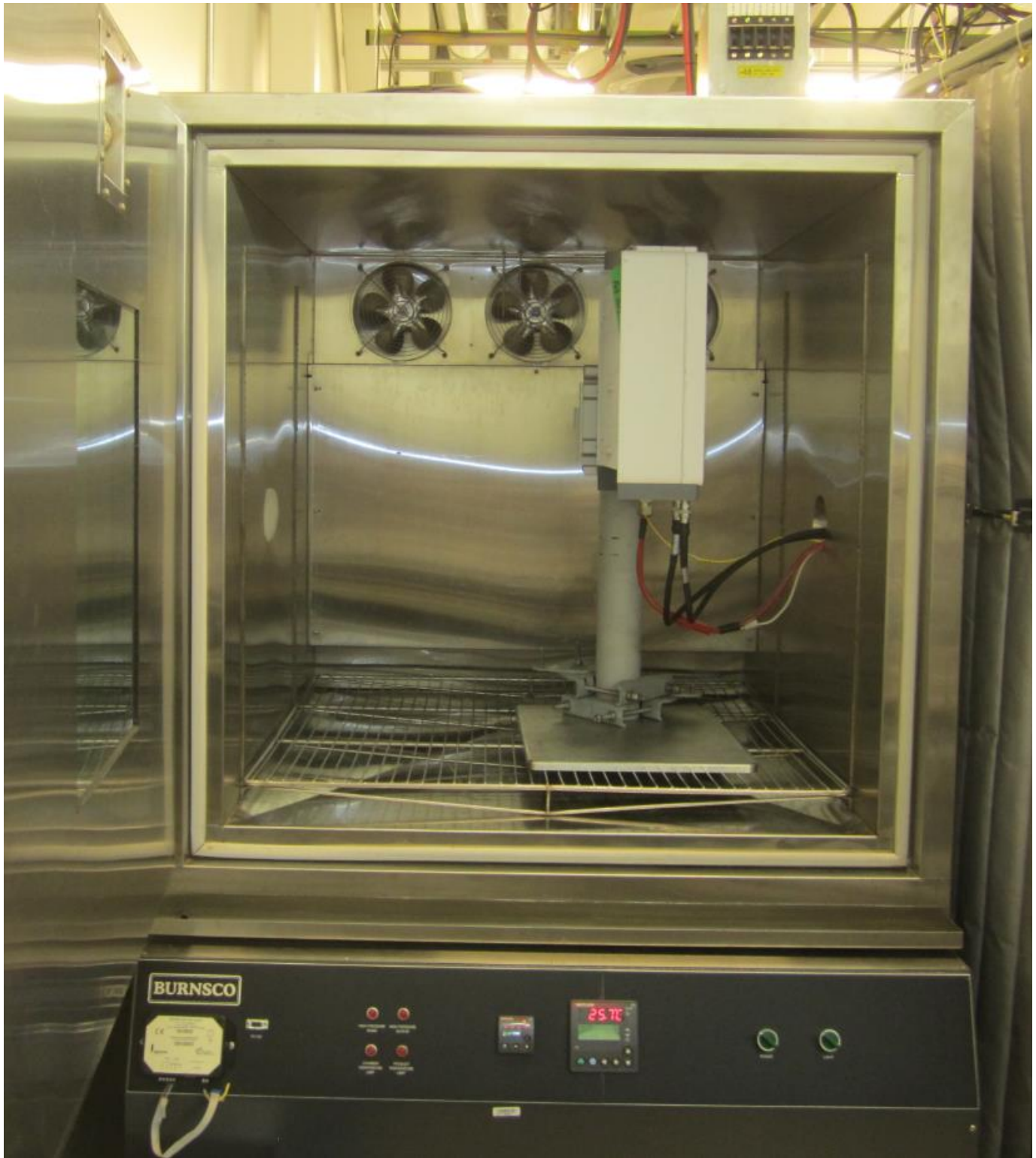
Figure 3.6-2: EUT Set-up for Radio Compliance Testing
