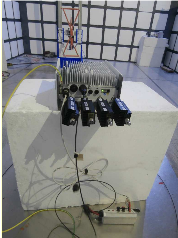
Radiated Emissions 30 MHz to 1 GHz
