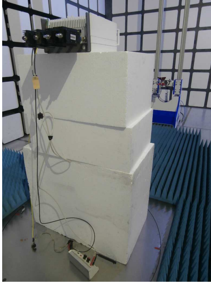
Radiated Emissions 1 GHz to 8 GHz
