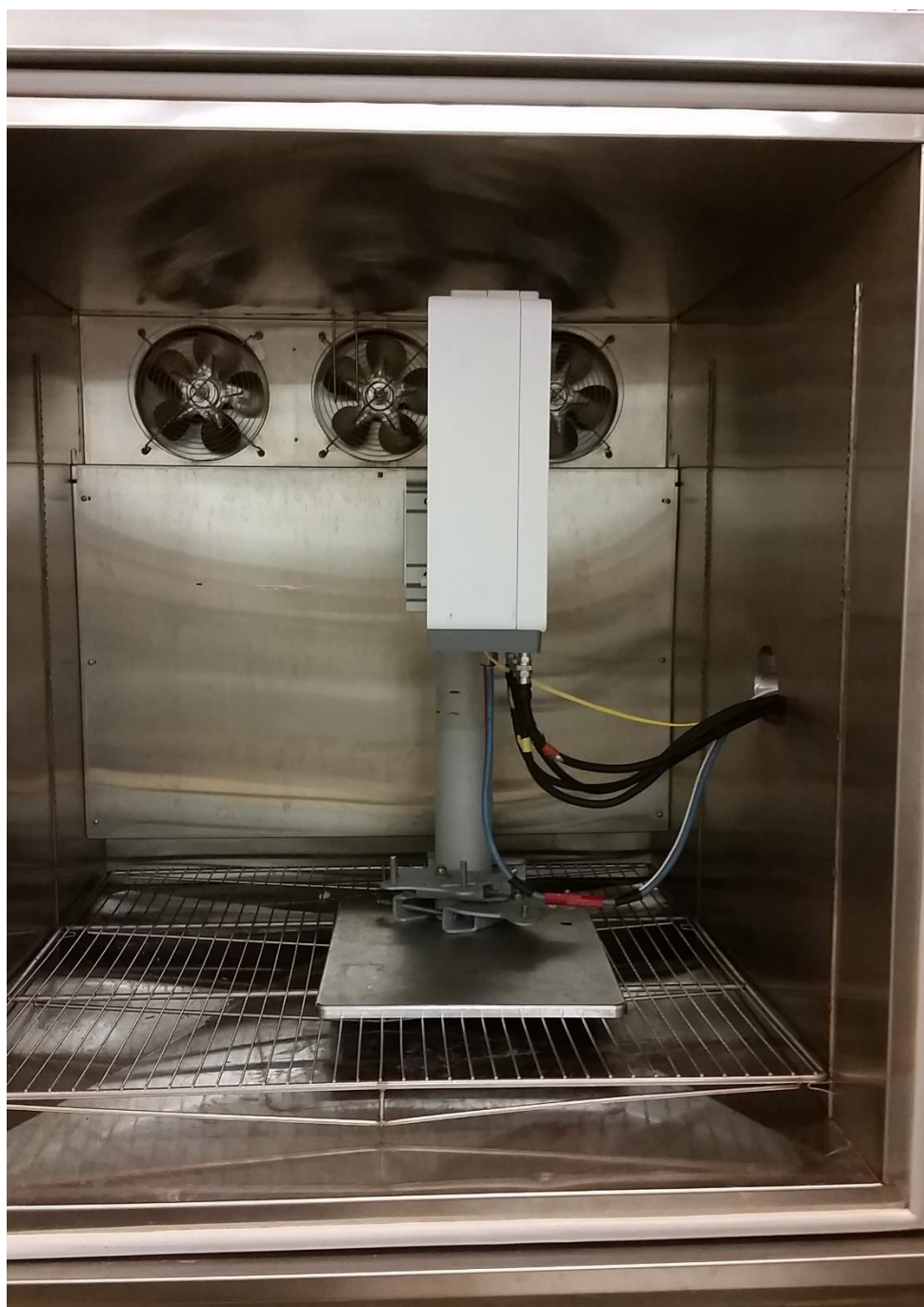
Figure 3.6-2: EUT Set-up for Radio Compliance Testing
