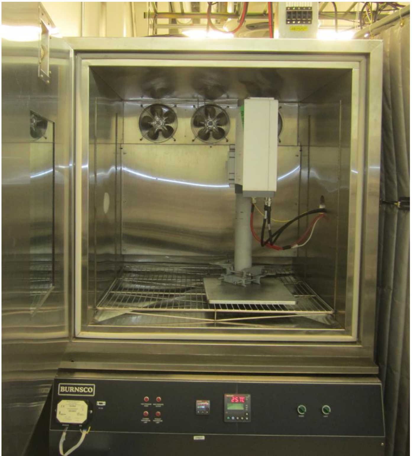
Figure 3.6-2: EUT Set-up for Radio Compliance Testing
