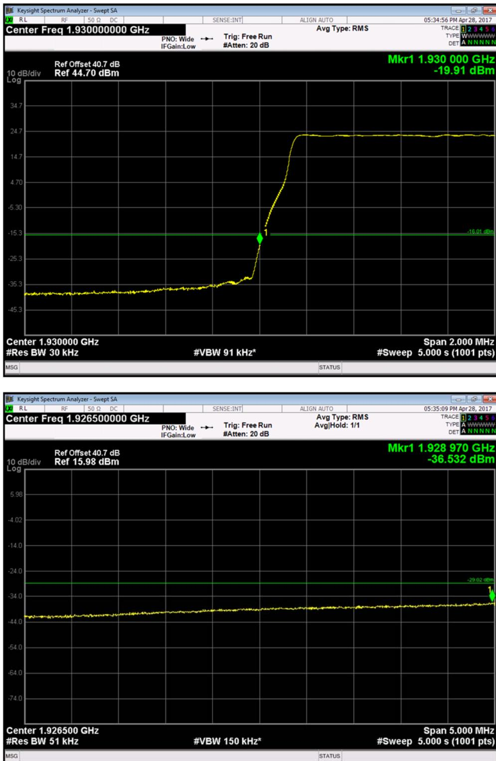
Channel Position  $T_{RFBW}$  - QPSK / Bandwidth 3.0 MHz
