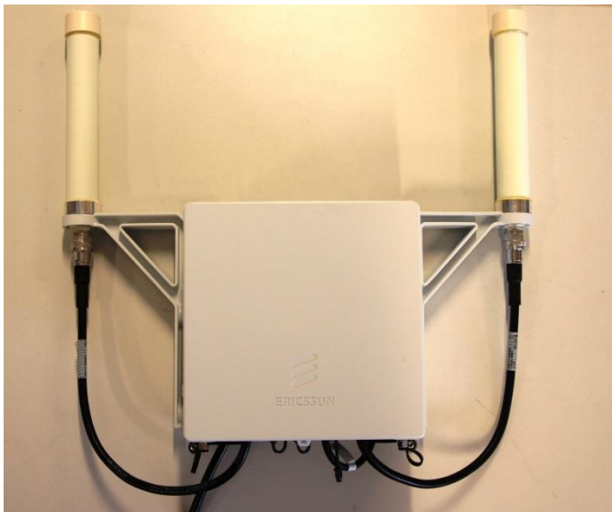
Front side with omni antenna KRE 101 2233/1
